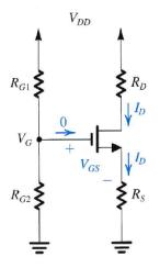
4. Design the circuit shown below so that the transistor operates in saturation with  $V_D$  biased 1 V from the edge of the triode region, with  $I_D = 1$  mA and  $V_D = 3$  V for each of the following two devices (use a 10-µA current in the voltage divider):
