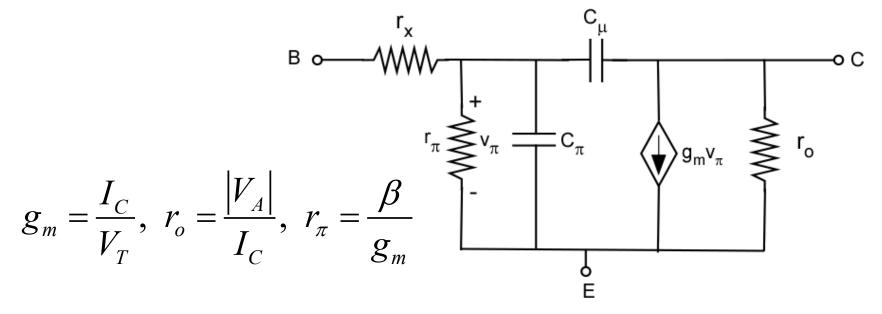
$$C_{\pi} + C_{\mu} = \frac{g_{m}}{2\pi f_{T}}, \quad C_{\pi} = C_{de} + C_{je}, \quad C_{de} = \tau_{F} g_{m}$$
