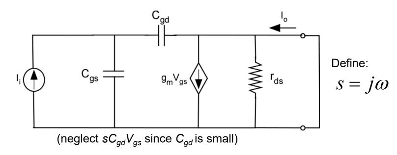
$$I_{o} = g_{m}V_{gs} - sC_{gd}V_{gs} \qquad \frac{I_{o}}{I_{i}} = \frac{g_{m}}{s(C_{gs} + C_{gd})}$$
