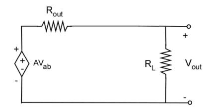
$$A_{MB} = \frac{v_{out}}{v_{in}} = \frac{R_{in}}{R_g + R_{in}} A \frac{R_L}{R_{out} + R_L}$$
