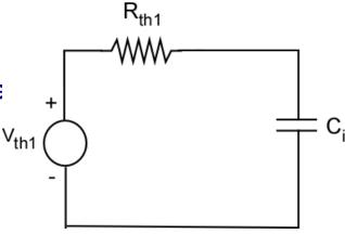
$$V_{th1} = \frac{v_{in}R_{in}}{R_g + R_{in}}$$
