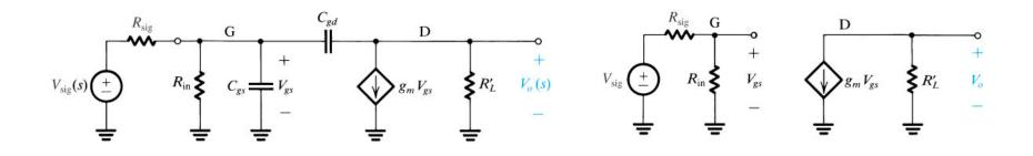
$$A_{M} = \frac{V_{o}}{V_{sig}} = -\frac{R_{in}}{R_{in} + R_{sig}} \left( g_{m} R_{L}^{'} \right) = -\frac{420}{420 + 100} \times 4 \times 3.33 = -10.8$$
