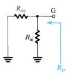
$$R_{gs} = R_{in} || R_{sig} = 420 k\Omega || 100 k\Omega = 80.8 k\Omega$$
