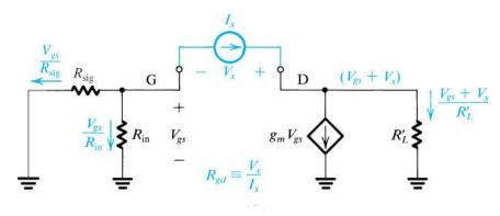
$$I_{x} = -\frac{V_{gs}}{R_{in}} - \frac{V_{gs}}{R_{sig}}$$
