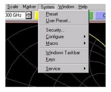
Now input your frequency range of interest, you can either go to Channel > Start/Stop and enter your start/stop frequencies or just use the Stimulus toolbar. You can also input the frequency range by defining its Center and Span.
