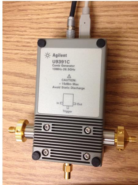
Figure 3: Repeated Pulse Generator Serves as a Phase Reference for NVNA Measurement System
