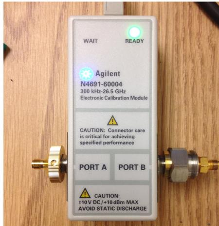
Figure 6: Electronic Calibration Module Used for Vector Error Correction
