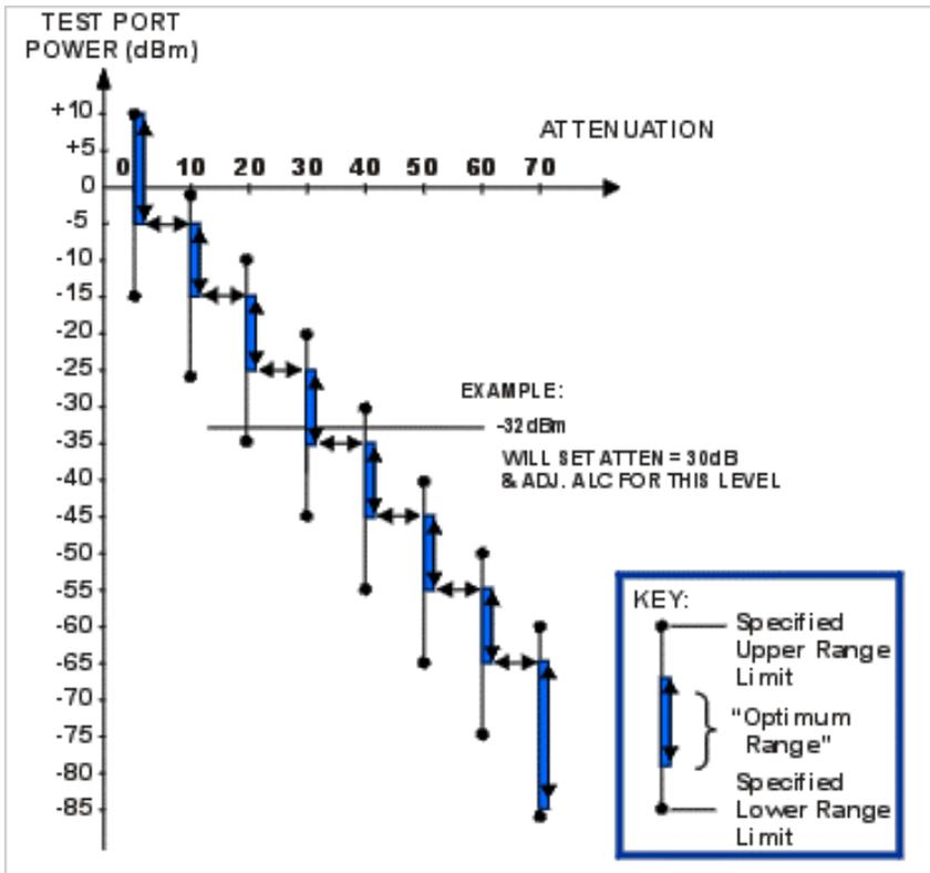
**Note:** Error correction is fully accurate only for the power level at which a measurement calibration was performed. However, when changing power within the same attenuator range at which the measurement calibration was performed, ratioed measurements can be made with nearly full accuracy (non-ratioed measurements with less accuracy).
