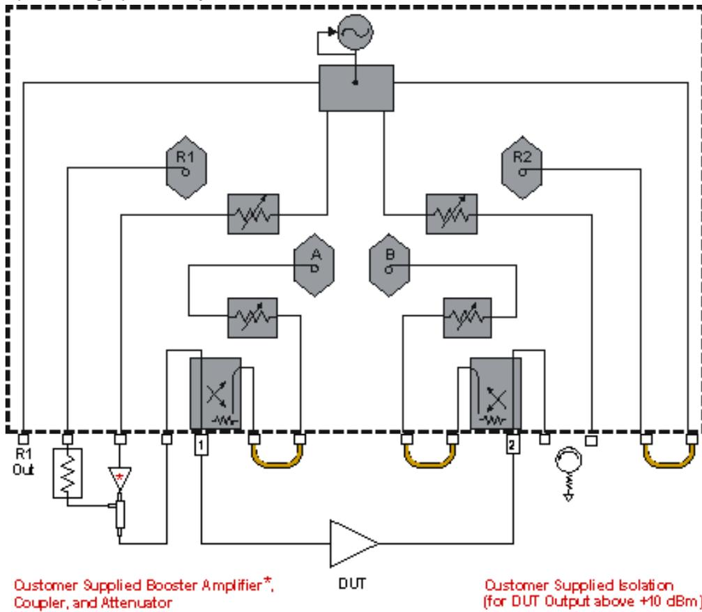
**Diagram: (E835xA, Option 015) Configuration for High-Power Measurements in both Forward & Reverse Directions**
