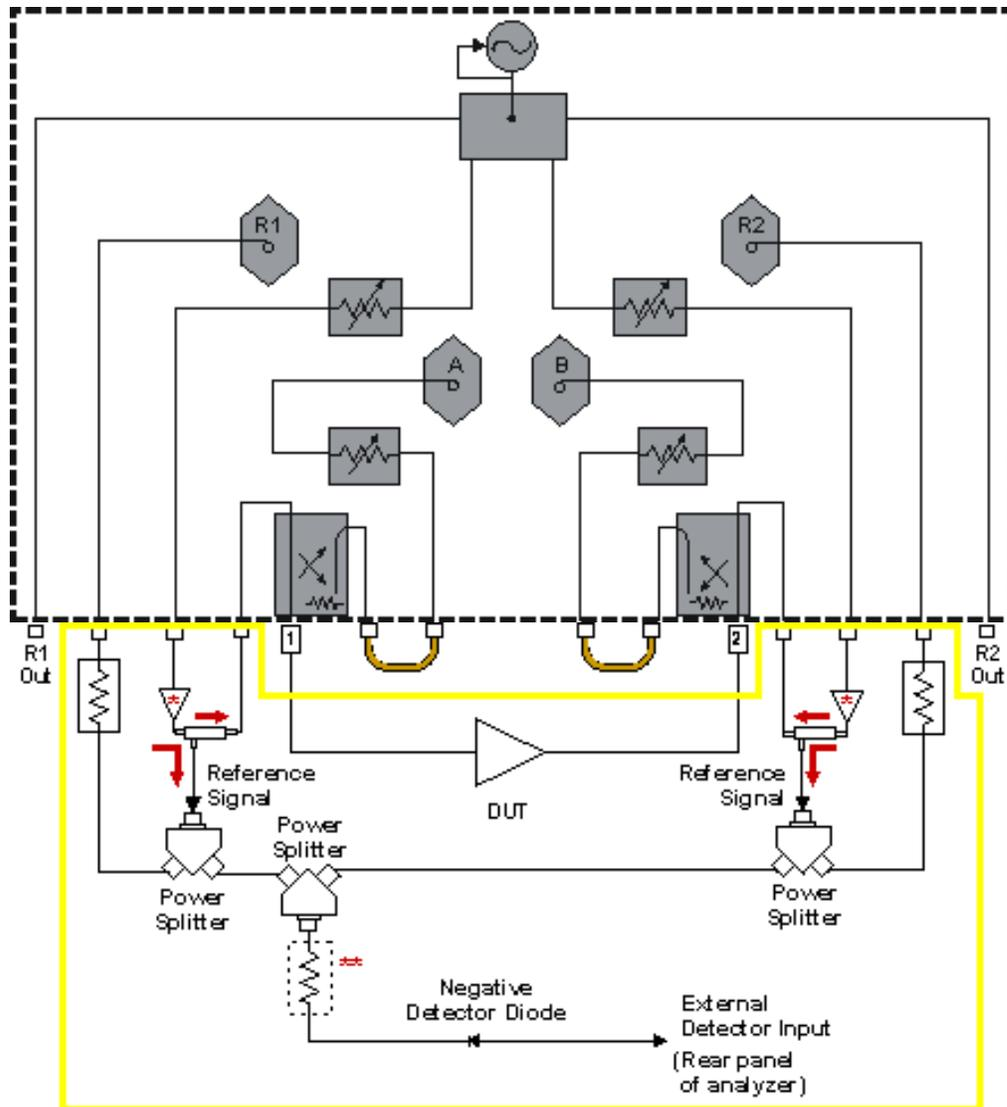
Customer Supplied Booster Amplifiers \*, Negative Detector Diode, Couplers, Power Splitters and Attenuators
