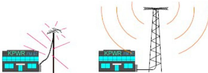
The radio station on the right installed properly "matched" transmission line and antenna. Very little of the transmitted signal is reflected, resulting in increased broadcast power, more listeners, more advertising revenue, and more profit. The amplifier, transmission, and antenna all need to be measured to ensure that reflected power is minimized.
