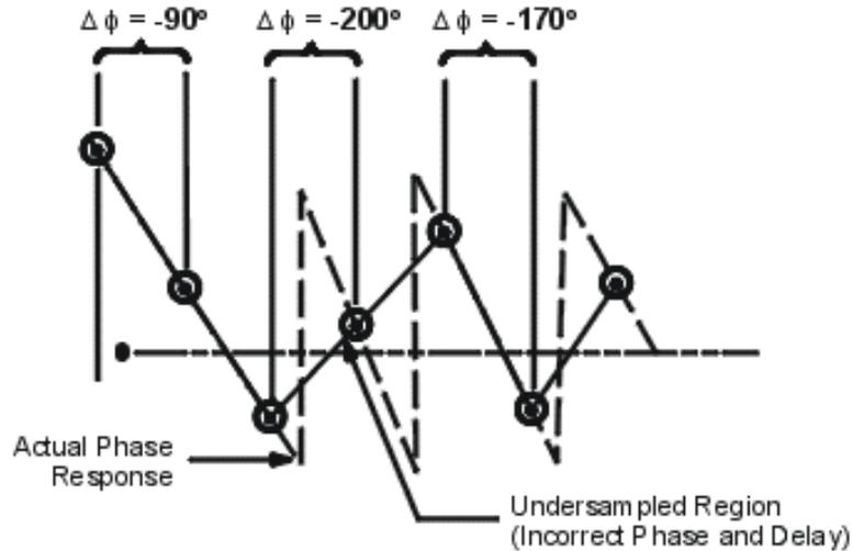
The frequency response is the dominant error in a group delay test setup. Performing a thru-response measurement calibration significantly reduces this error. For greater accuracy, perform a 2-port measurement calibration.
