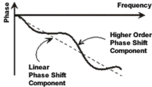
$$\begin{aligned} \text{Group Delay} = t_g &= \frac{-d\phi}{d\omega} && \phi \text{ in Radians} \\ &&& \omega \text{ in Radians/Sec} \\ &= \frac{-1}{360^\circ} \cdot \frac{d\Theta}{df} && \Theta \text{ in Degrees} \\ &&& f \text{ in Hz } (\omega = 2\pi f) \end{aligned}$$
