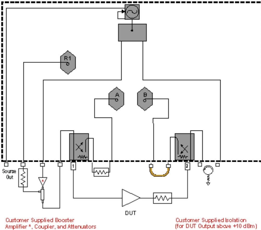
**Diagram: (E880xA, Option 014) Configuration for High-Power Measurements in both Forward and Reverse Directions**
