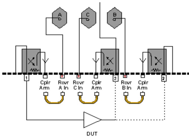
\* Measure the receiver input power where your external circuitry connects here.
