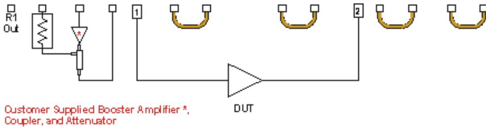
**Diagram: (E835xA, Option 015) Configuration (with an Isolator) for High-Power Measurements in the Forward Direction**
