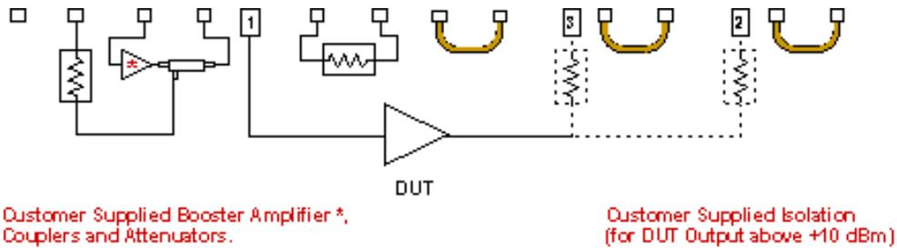
**Diagram: (N338xA, Option 014) Configuration (with an Isolator) for High-Power Measurements in the Forward Direction**
