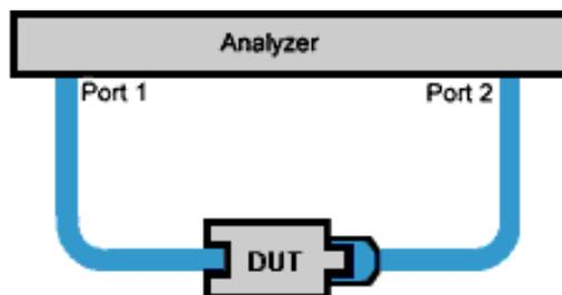
When calibrating for an insertable device, the test ports at your measurement reference plane connect directly together. This is called a zero-length thru. That means the definition, or electrical description the analyzer uses in the calibration process, has zero-length: no delay, no loss, no capacitance, and no inductance.
