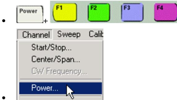
**Note:** If Power Sweep is selected, (from Sweep Type dialog box) clicking **Channel, Power** will invoke a Power (Sweep) dialog box.
