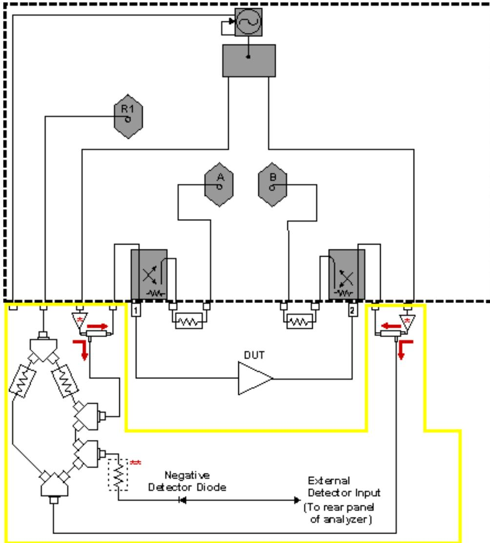
\*\* This attenuator may be required to meet the recommended power level input ( +10dBm to -20dBm ) of the detector diode.
