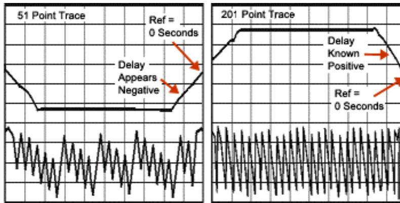
**Tip:** To check if aliasing might be occurring in a measurement, either increase the number of points or reduce the frequency span.
