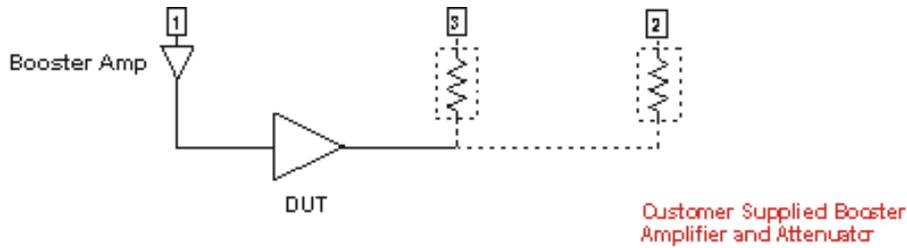
**Diagram: (N338x) Configuration for Non-Boosted High-Power Measurements in both Forward and Reverse Directions**
