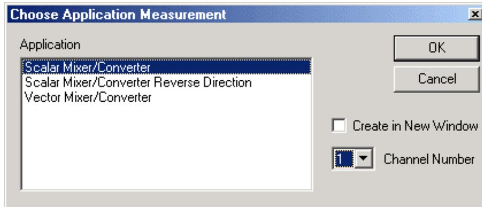
**Note:** Each of these three measurements must be created in a separate channel. They can NOT share the same channel.
