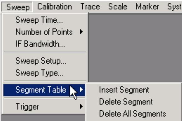
**Insert Segment** - adds a sweep segment before the selected segment.
