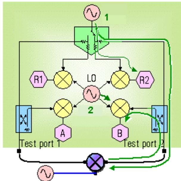
1: Internal source tuned to DUT input
