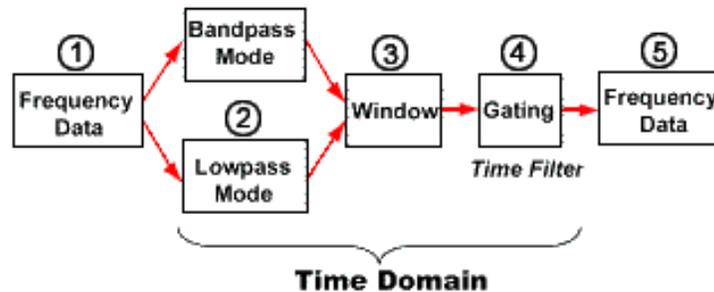
1. **Frequency Data** -- is collected when the analyzer measures a device response in the frequency domain.
