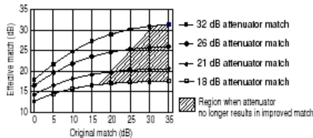
The larger the attenuation, the more nearly the resulting match approaches that of the attenuator, as shown in the following graphic. However, excessive attenuation is not desired because that will decrease the dynamic range of the measurement system.
