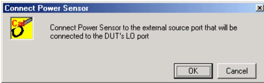
This means: Connect the power sensor to the external source connector at the point where it mates to the input of the mixer (after cables and other components).
