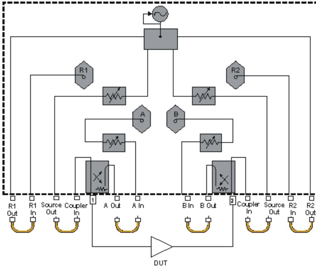
**Diagram: (E835xA, Option 015) Configuration for High-Power Measurements in the Forward Direction**
