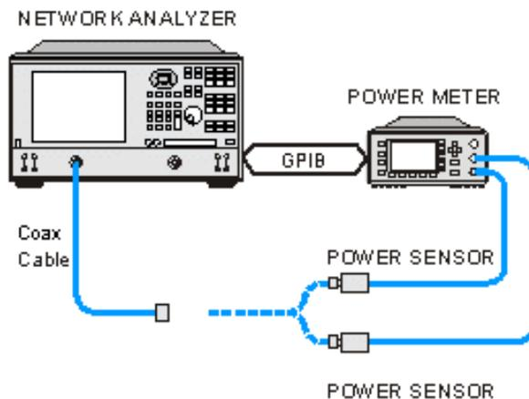
**Note:** You can use the 82357A USB/GPIB Interface to control the power meter.
