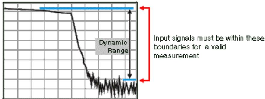
To help reduce measurement uncertainty, the analyzer dynamic range should be greater than the response that the DUT exhibits. For example, measurement accuracy is increased when the DUT response is at least 10 dB above the noise floor. The following methods can help you increase the dynamic range.
