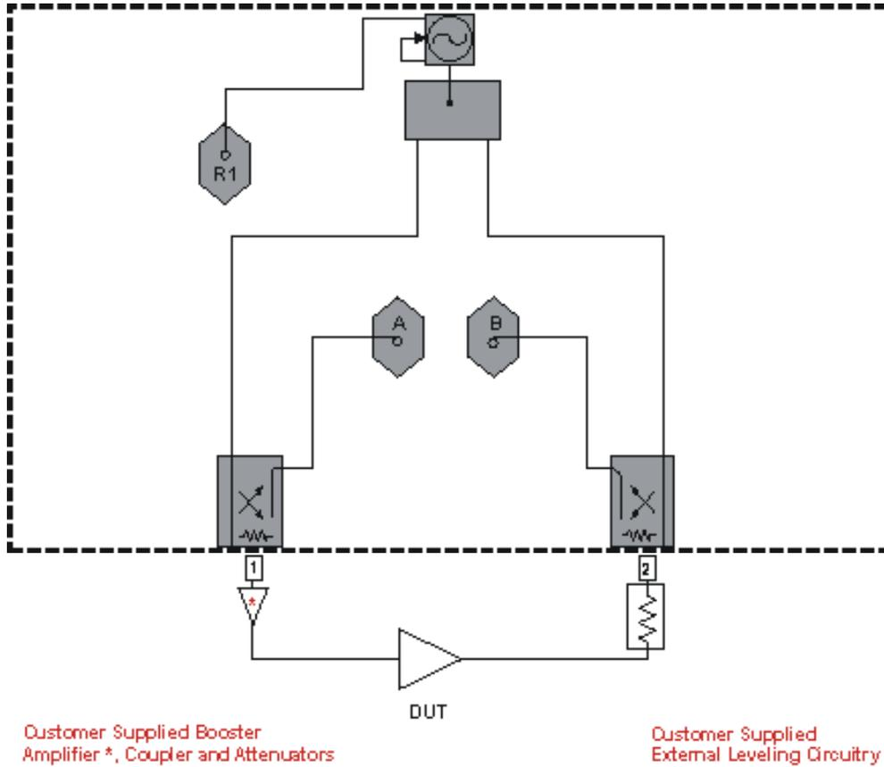
**Diagram: (E880xA) Configuration for Non-Boosted High-Power Measurements in both Forward and Reverse Directions**
