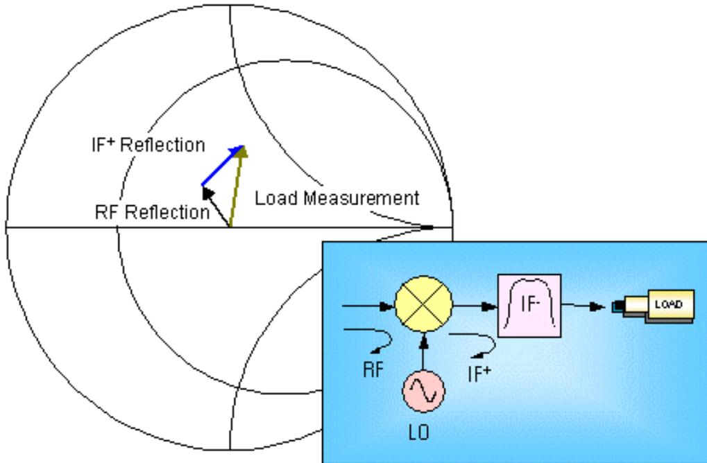
This vector plot shows how the terms combine to make the load measurement. Since  $\Gamma_{\text{Termination}} = 0$  for a load, there is no IF- term, and no fourth term associated with the  $S_{22} * \Gamma_{\text{Termination}}$ .
