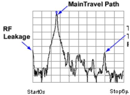
**Tip:** To see the response of just the SAW filter main path, you can set the gate to block all but the main pulse. Then in the frequency domain, only the frequency response of the main path is displayed.
