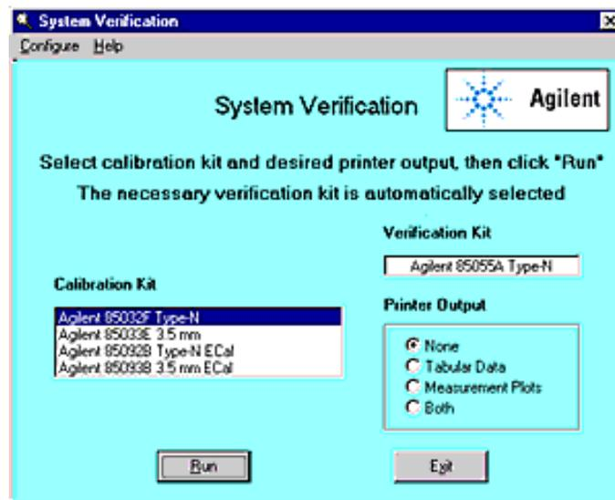
4. In the **Calibration Kit** box, select the calibration kit that is being used. The corresponding verification kit to use appears in the **Verification Kit** box.
