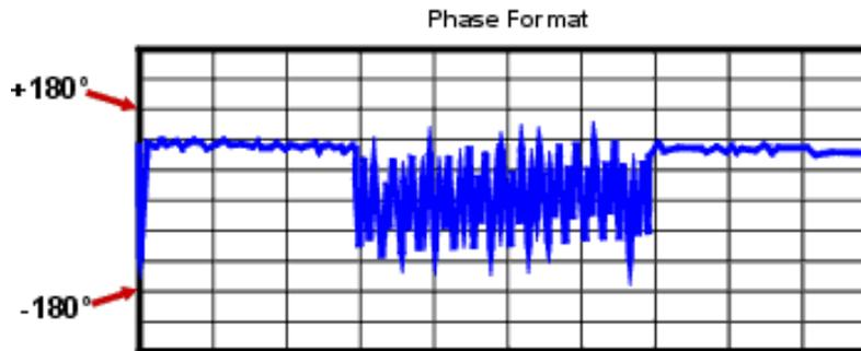
The sawtooth pattern does not always reach  $+180$  degrees and  $-180$  degrees. This is because the measurement is made at discrete frequencies, and the data point at  $+180$  degrees and  $-180$  degrees may not be measured for the selected sweep.
