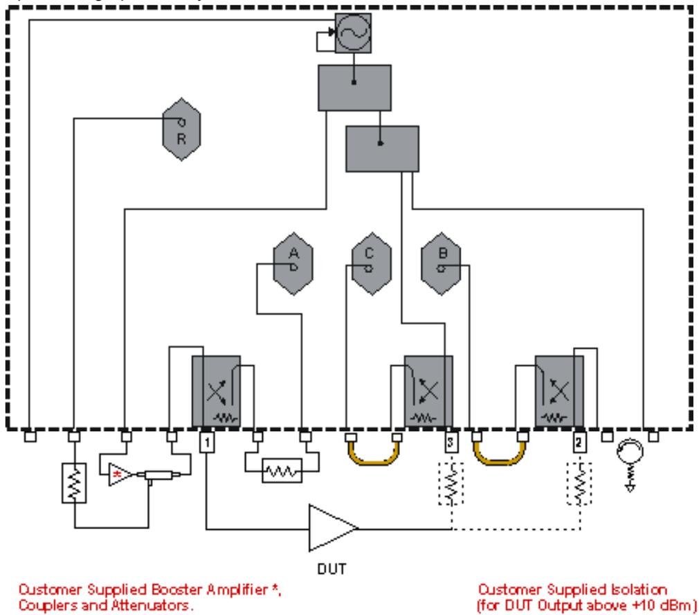
**Diagram: (N338xA, Option 014) Configuration for High-Power Measurements in both Forward and Reverse Directions**
