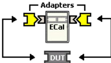
2. Either perform a Guided calibration using mechanical standards or recall a Cal Set. This is required to make accurate measurements of the ECAL module and adapters.
