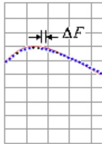
$$\Delta F = \frac{\text{Frequency Span}}{\# \text{ of Points} - 1}$$
