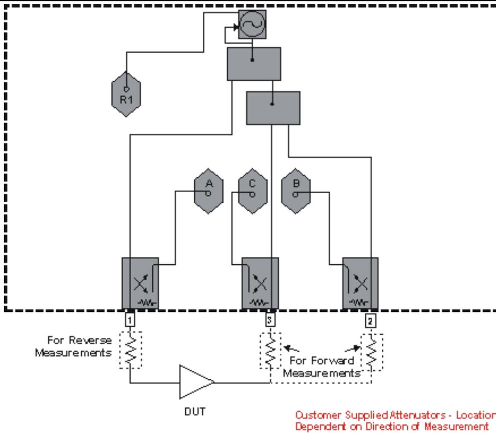
**Diagram: (N338x) Configuration using a Booster Amplifier**
