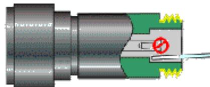
5. Let alcohol evaporatethen use compressed air to blow surfaces clean.
