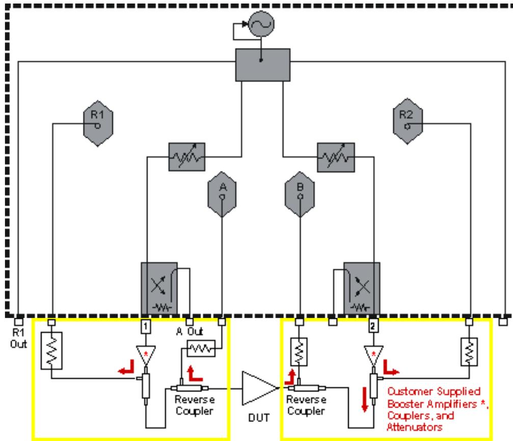
**Diagram: (E835x) External Leveling using One Booster Amplifier**
