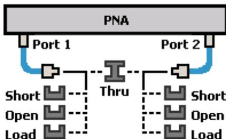
3. Measure the ECal module, including adapters, as though it were a DUT.
