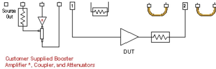
**Diagram: (E880xA, Option 014) Configuration (with an Isolator) for High-Power Measurements in the Forward Direction**
