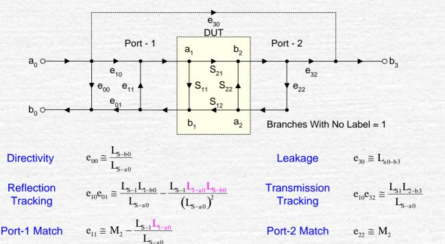
There are also Errors caused by the Converter, IF, Cables and Connectors
