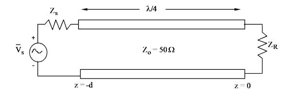
5. For the above figure, let  $\overline{V}_s = 1$  volt,  $Z_s = 30 \Omega$ , and  $Z_R = 40 \Omega$ .
