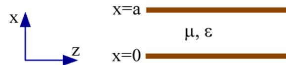
**$a$**  is the distance separating the two PEC plates
