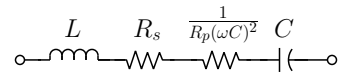
Figure 3.10: Equivalent series RLC circuit of a capacitor, valid where R_p \gg 1/(\omega C) , derived from the model shown in Figure 3.9.
