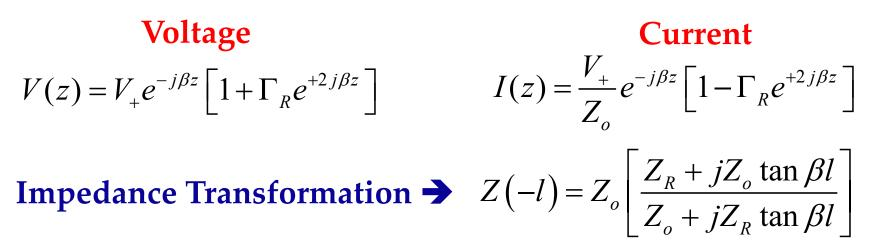
**Reflection Coefficient Transformation**  $\rightarrow \Gamma(-l) = \Gamma_R e^{-2j\beta l}$
