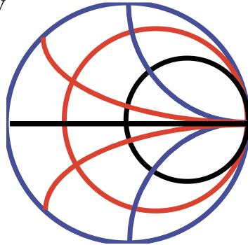
Thus, going from normalized impedance to normalized admittance corresponds to a 180 degree shift.
