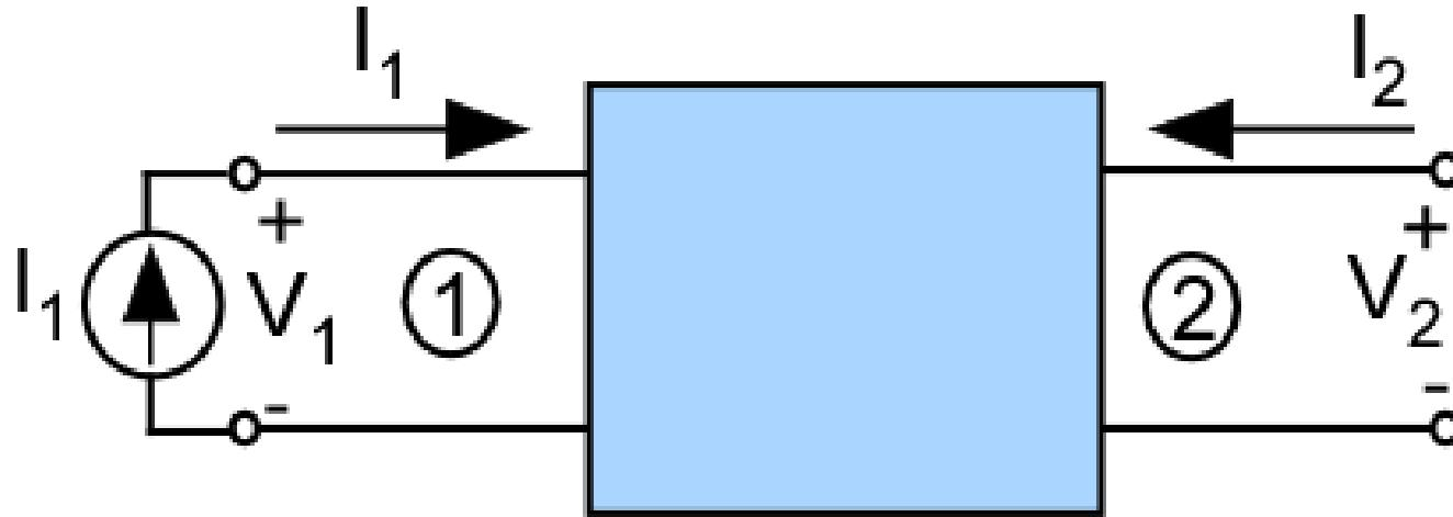
$$z_{11} = \left. \frac{V_1}{I_1} \right|_{I_2=0}$$
