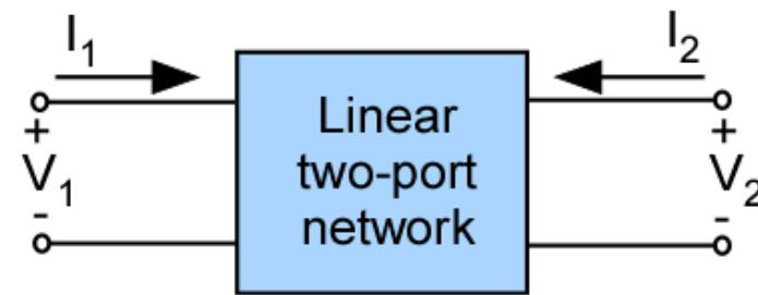
Relationship with Z parameters is obtained by first expressing ABCD parameters in terms of Z parameters
