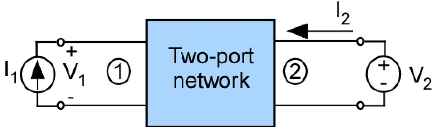
$$V_1 = h_{11}I_1 + h_{12}V_2$$
