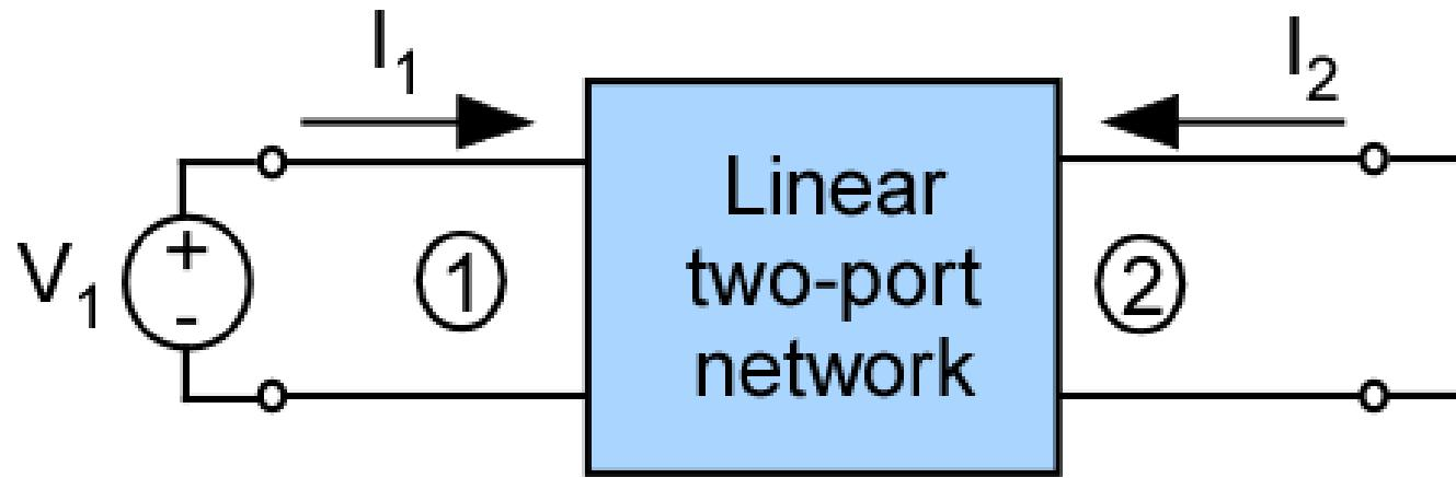
$$y_{11} = \frac{I_1}{V_1} \Big|_{V_2=0}$$
