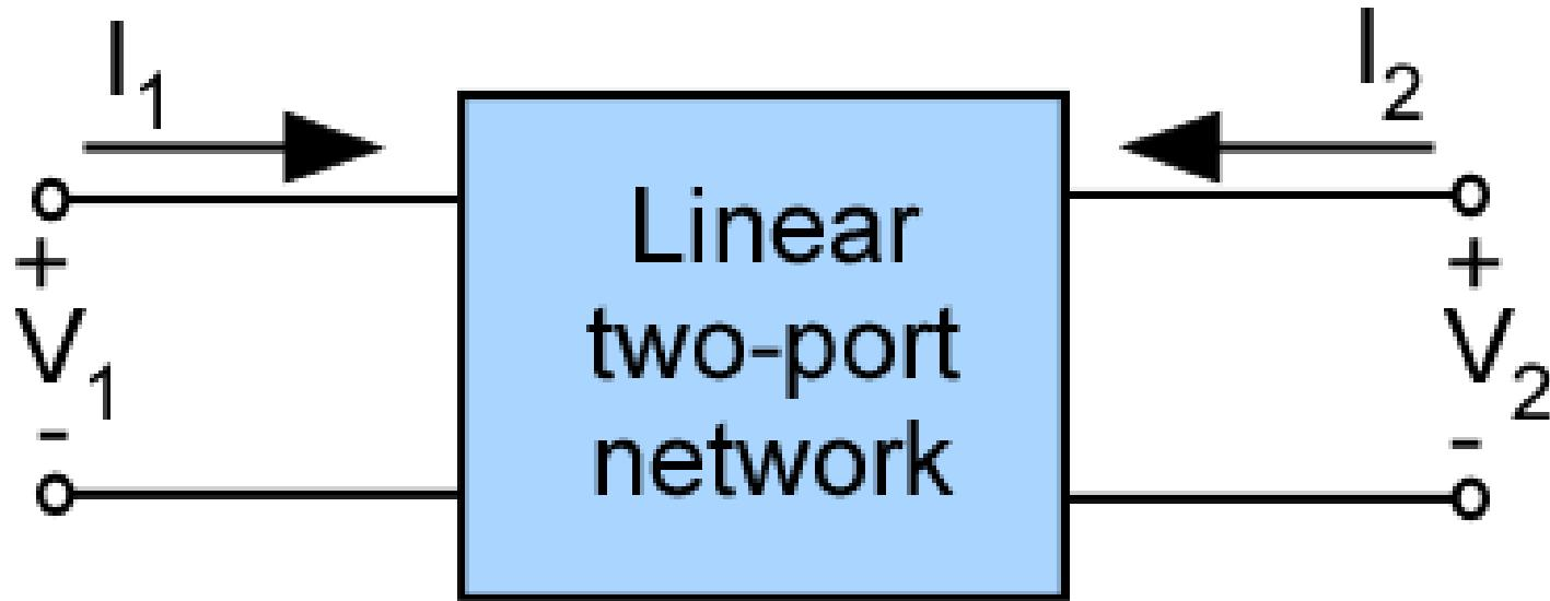
Use a two-terminal representation of system for input and output
