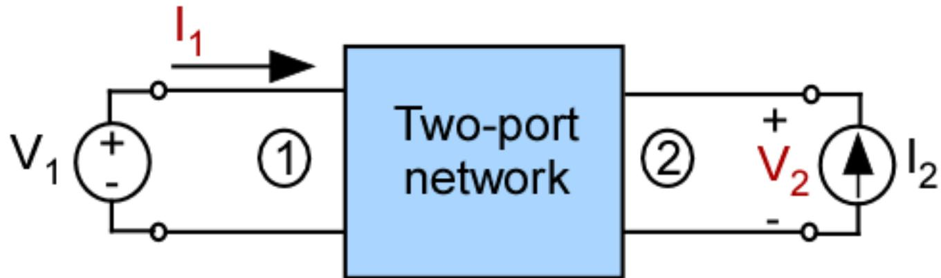
$$I_1 = g_{11}V_1 + g_{12}I_2$$
