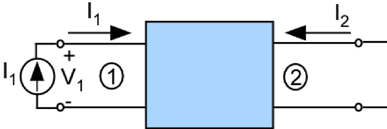
$$h_{11} = \frac{V_1}{I_1} \Big|_{V_2=0}$$
