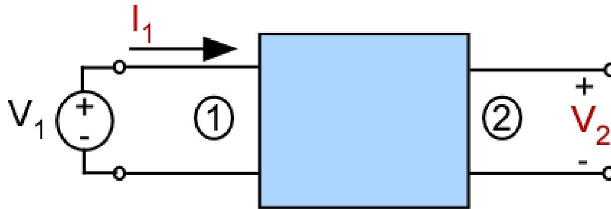
$$g_{11} = \left. \frac{I_1}{V_1} \right|_{I_2=0}$$
