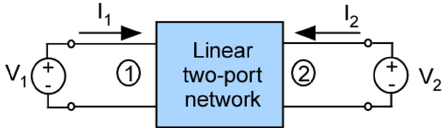
$$I_1 = y_{11}V_1 + y_{12}V_2$$
