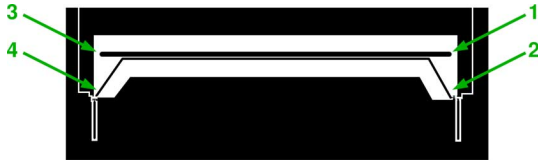
Fig. 11. Layout of PCB with coupled interconnect structure under investigation. Port numbering is also specified.
