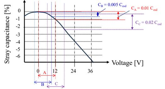
Fig. 5. Bias-voltage dependencies of stray capacitance of ESD protection device with three different bias conditions.
