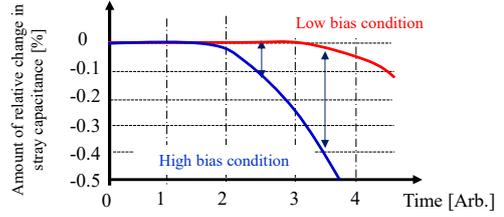
Fig. 4. Time dependencies of stray capacitance change of ESD protection device
