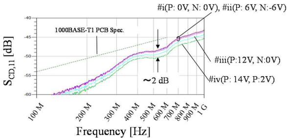
Fig. 10. Experimental results of MCL under different voltage-bias conditions
