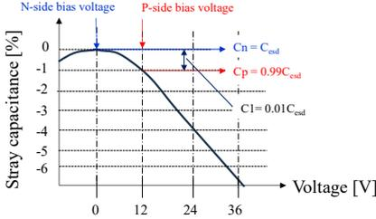
Fig. 3. Bias-voltage dependencies of stray capacitance of ESD protection device
