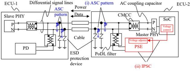
Fig. 2. Circuit composition of PoDL communication with proposed active-mode-conversion-noise suppressor (AMCNS).
