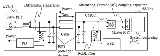
Fig. 1. Circuit composition of conventional power over data line (PoDL) communication
