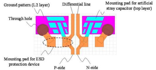
Fig. 6. Designed ASC pattern for evaluation board
