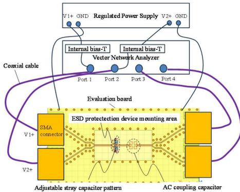
Fig. 9. Measurement setup for IPSC using evaluation board
