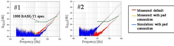
Fig. 7. Experimental results of mode conversion loss (MCL),  $S_{cd,11}$ , using evaluation board
