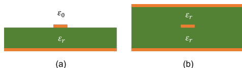
Fig. 1. Cross-section view of (a) microstrip and (b) Stripline.
