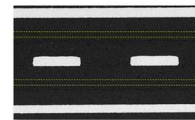
Fig. 2. A cross-section illustration of the skip-layer design. Yellow dash lines indicate the voided (“skipped”) metal layers.
