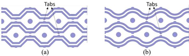
Fig. 5. Tabbed pin area wiring (a) Zigzag (b) Arc
