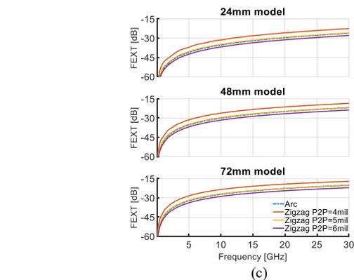
Fig. 4. (a) PCB Misregistration schematic (b) HFSS arc model top view with misregistration (c) FEXT with misregistration
