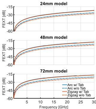
Fig. 6. FEXT for tabbed pin area wiring with misregistration
