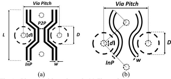
Fig. 1. Pin area wiring schematic (a) Zigzag (b) Arc
