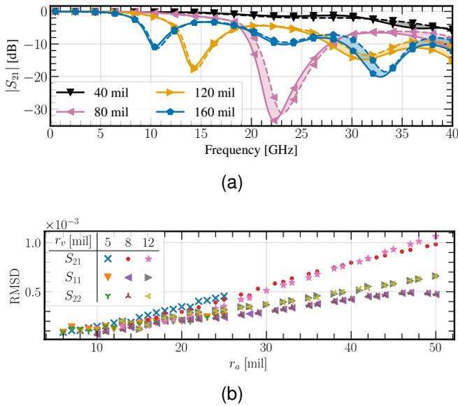
Fig. 4. Correlation results for the setup shown in Fig. 1b. (a) shows  $S$ -parameters for different distances to the ground fence. Continuous lines represent PB and dashed lines FW results, respectively. (b) shows a steady increase of RMSD for different antipad radii.
