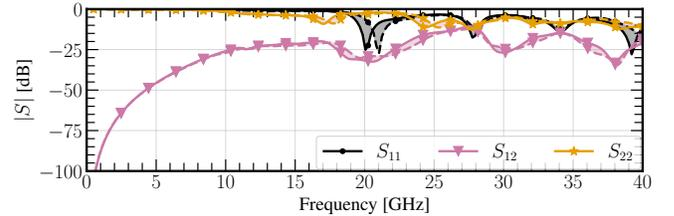
Fig. 3. Reflection and near end crosstalk for the structure of Fig. 1a showing agreement between the two simulation methods. Continuous lines represent PB and dashed lines FW results, respectively.
