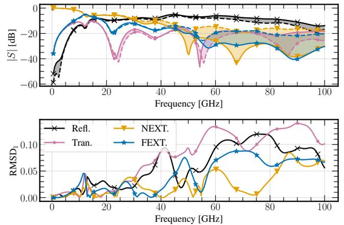
Fig. 5. Transmission, reflection, near and far end crosstalk are plotted over frequency. Continuous lines represent PB and dashed lines FW results, respectively. The RMSD is calculated for each frequency ( $N = 1$ ) and plotted in the figure below. The legend is valid for both plots. An increase in RMSD between PB and FW results with higher frequency becomes apparent.
