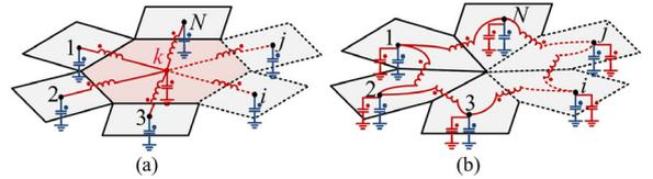
Fig. 3. Physics-inspired circuit transformation for absorbing an insignificant node . a) Meshes and circuit prior to transformation. b) Equivalent meshes and circuit posterior to transformation.
