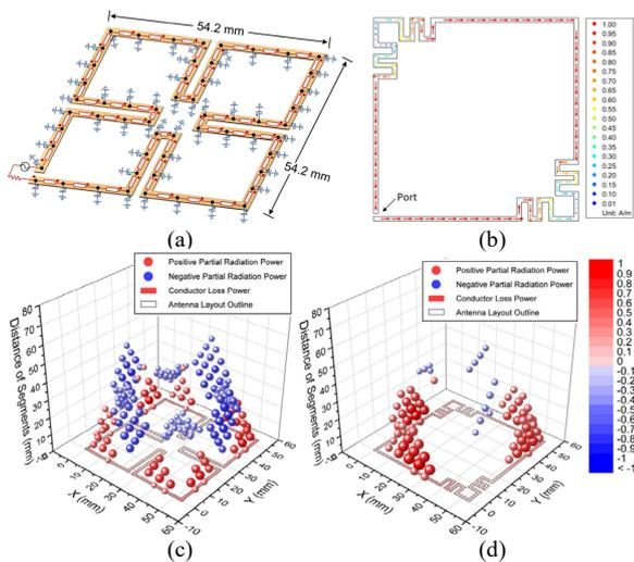
Fig. 4. Loop antenna structures and their holographic radiation diagram. a) loop antenna design 1. b) loop antenna design 2. c) holographic radiation diagram of design 1. d) holographic radiation diagram of design 2.
