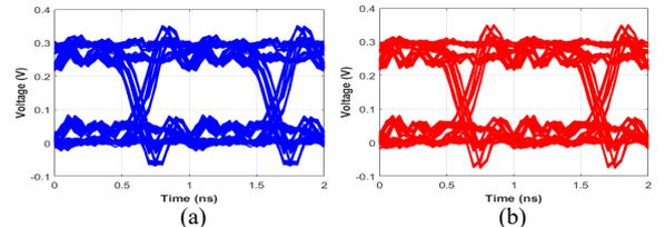
Fig. 2. Simulated eye-diagram obtained by PEEC and MMC. a) eye-diagram obtained by PEEC. b) eye-diagram obtained by MMC.
