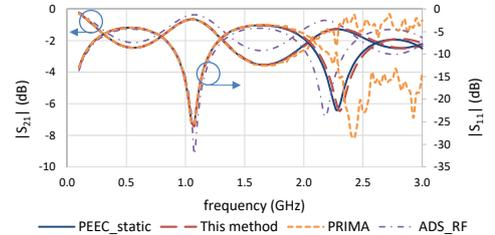
Fig. 1. Simulated S-parameter obtained by PEEC, MMC, PRIMA, and ADS software.
