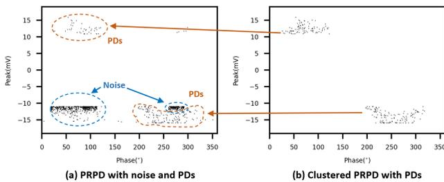
Fig. 3. Frequency feature based clustering for noise and PD signals separation.
