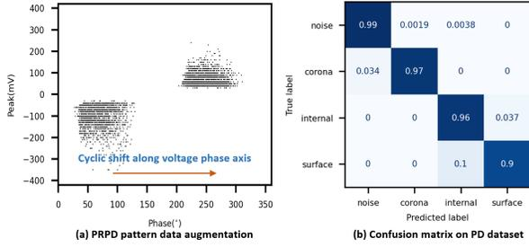
Fig. 4. (a) Demonstration of the data augmentation strategy of the PRPD pattern for deep neural network training. (b) Confusion matrix on the testing set achieved by the proposed method with knowledge distillation and multi-task feature learning.
