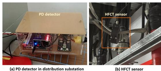
Fig. 1. The designed PD detector and high-frequency current transformer (HFCT) sensor deployed in distribution substation.
