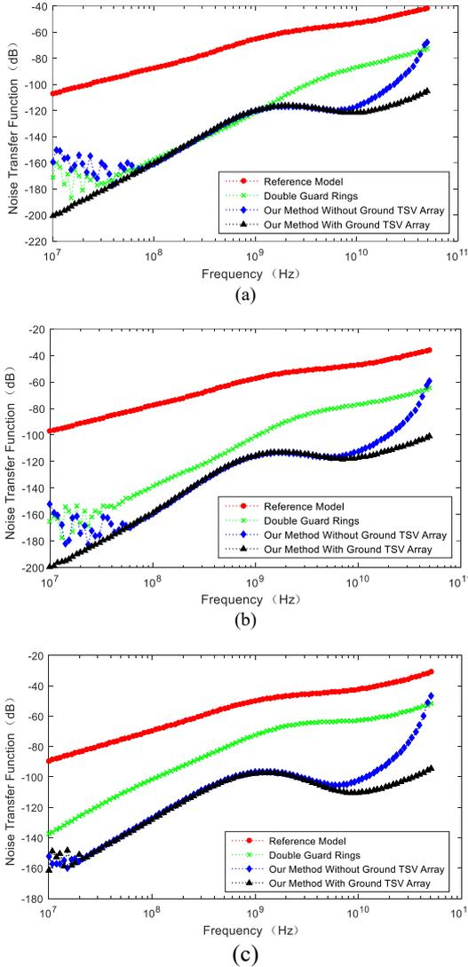
Fig. 3. Noise suppression performance comparison among the reference model, double guard rings, our previous method with only P+ contact array and grid ground plane, and our method with P+ contact array, grid ground plane and ground TSV array for three cases. (a) Pad-Pad, (b) Pad-TSV, (c) TSV-TSV.
