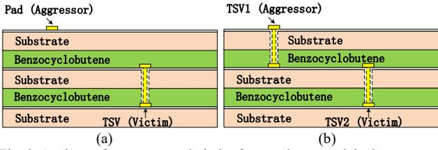
Fig. 2. Settings of aggressor and victim for two-layer model when considering the suppression of noise from (a) pad to TSV, and (b) TSV to TSV.
