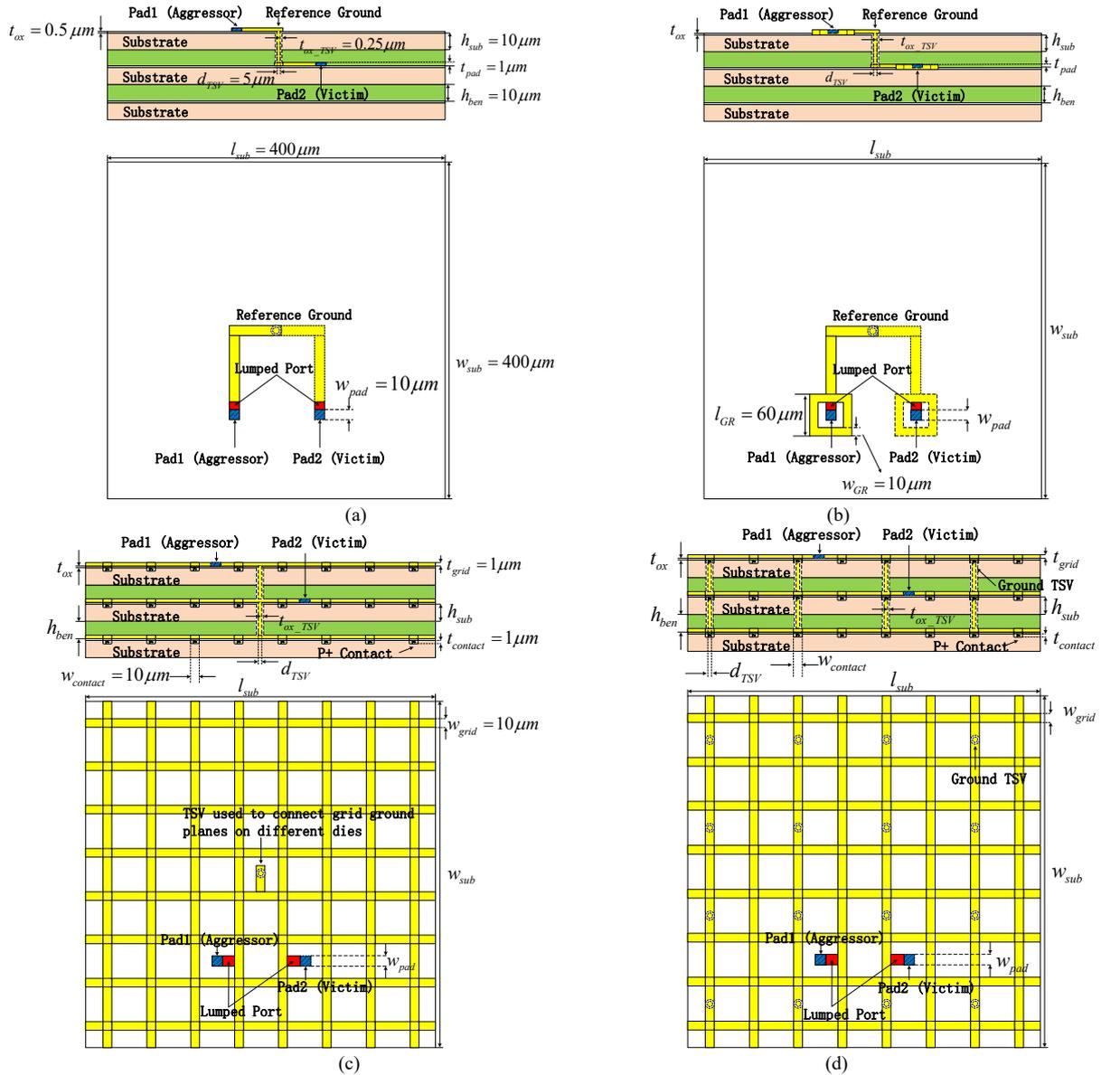
Fig. 1. Noise isolation methods for three-layer 3D SiP: (a) reference model, (b) double guard rings method, (c) our previous method without ground TSV array, (d) our method with ground TSV array. All the structures only shows the case of coupling noise isolation between pad and pad.
