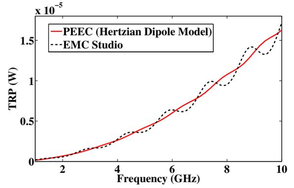
Fig. 7. TRP calculated with EMC studio and with the compensated geometry.
