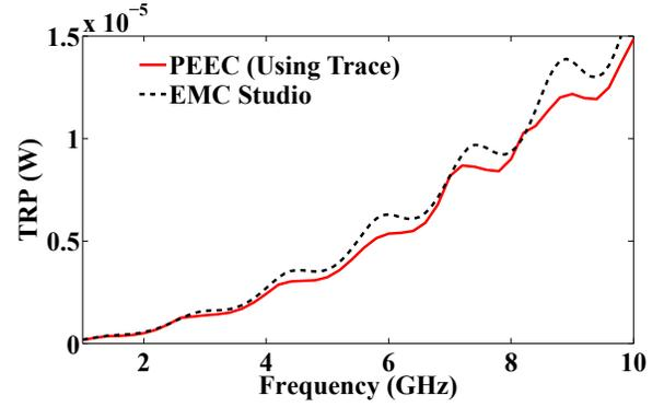
Fig. 4. TRP of the two wires.
