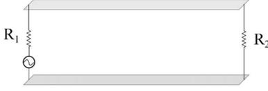
Fig. 1. Geometry of the two wires with a voltage source between the two wires.
