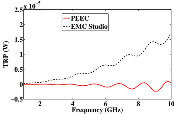
Fig. 2. (a) TRP of the two wires with a voltage source between the two wires calculated with PEEC. (b) TRP calculated with EMC studio [8].
