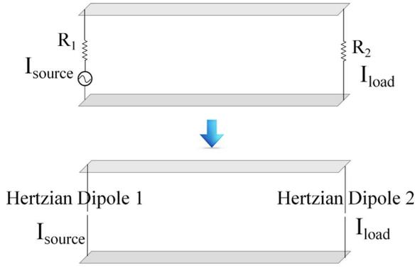
Fig. 5. Geometry of the two wires, and the compensation policy for the structure.
