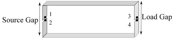
Fig. 3. Geometry of the two wires, with 1 V voltage source and 192.5  $\Omega$  internal impedance between node 1 and 2, and a 192.5  $\Omega$  load between node 3 and 4.
