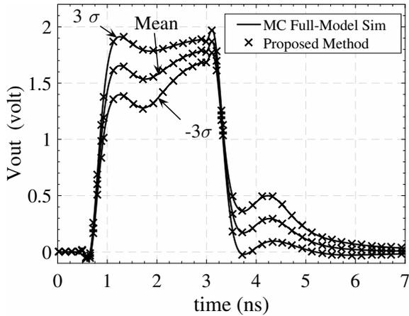
Fig. 2. Time-domain statistical analysis for the output voltage at the far end of line 1.
