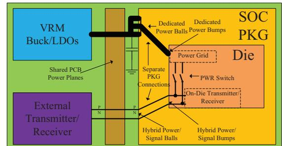
Fig. 1. High-level overview of the proposed PLC on PDN.
