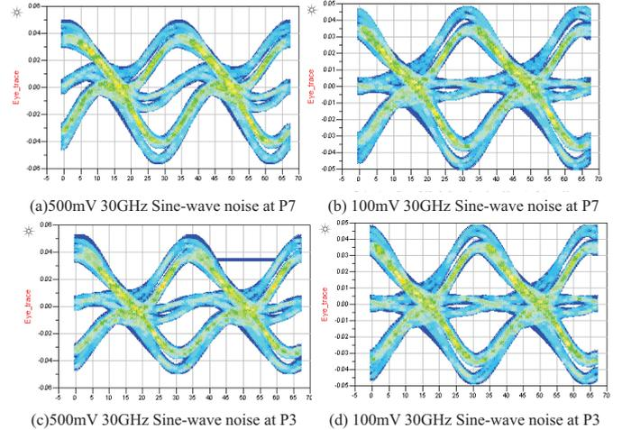
Fig. 8. Receiver eye diagram after equalization with near-end and far-end noise source from power plane.
