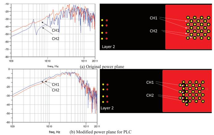
Fig. 4.  $S_{dd21}$  of two channels from the original and the modified power plane.
