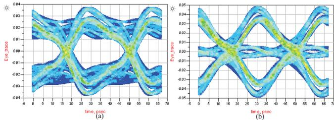
Fig. 6. Eye diagram of a 30GHz PLC (a) without equalizer, (b)with equalizer.
