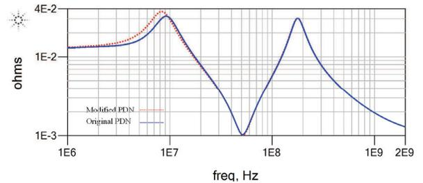
Fig. 9. Impedance profile for the original and the modified PDN with a pair of PLC
