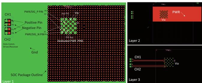
Fig. 3. An overview of the 4-layer PCB test coupon layout for PLC.
