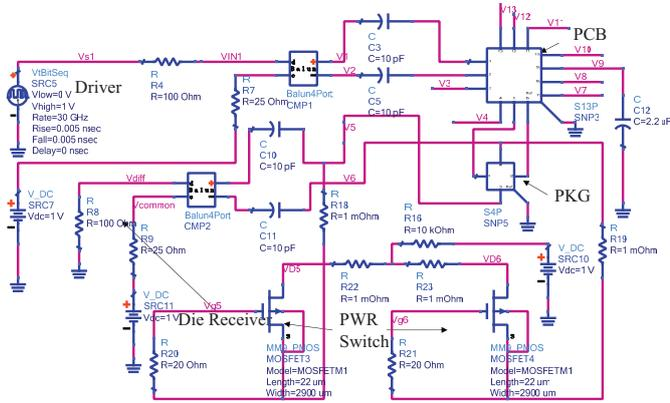
Fig. 5. Schematic for data communication on a PDN
