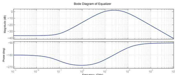
Fig. 7. The transfer function of the receiver equalizer.
