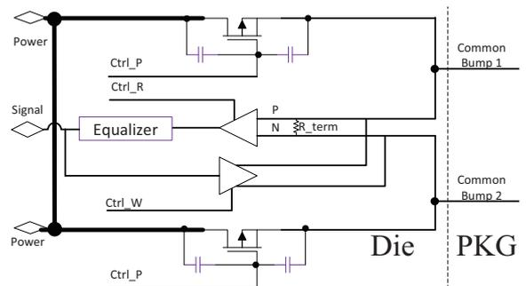
Fig. 2. The circuit diagram of a on-die differential signal-to-power switch
