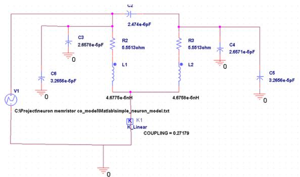
Figure 5: Two MIVs SPICE Model with One Layer Memristor
