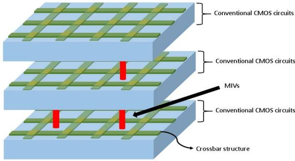
Figure 1: 3D-IC Neuromorphic Structure using MIVs
