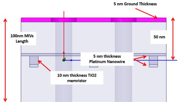
Figure 3: Side View of Q3D Extractor Model of Integration between MIVs and Memristor-based Crossbar Structure
