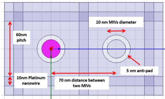
Figure 2: Top View of Q3D Extractor Model of Integration between MIVs and Memristor-based Crossbar Structure
