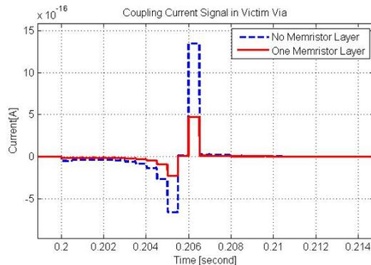
Figure 7: Comparison of Current Coupling Signal Waveform Victim MIV between No Memristor and One Memristor Case
