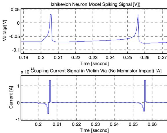
Figure 6: Spiking Stimulus Signal Waveform and its Current Coupling Signal Waveform on Victim MIV
