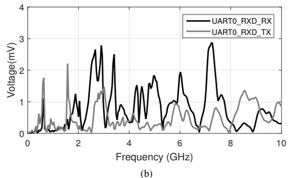
Fig. 4. (a) Intel Galileo board illuminated by a 1-V/m plane wave polarized in the  $\bar{\theta}$  direction with an incident direction in  $\phi = 45^\circ$ ,  $\theta = 30^\circ$ , (b) voltages induced at the two ports on the signal net UART0\_RXD.
