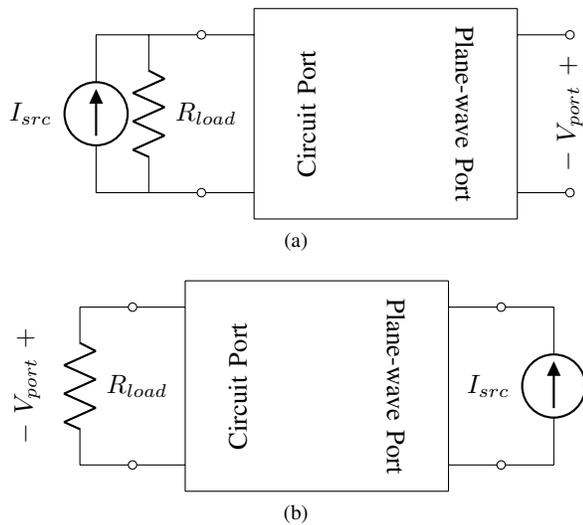
Fig. 1. Circuit diagram of (a) the forward radiation problem and (b) the reverse problem.
