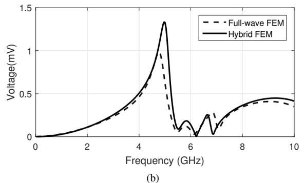
Fig. 2. (a) A microwave filter illuminated by a 1-V/m plane wave polarized in the +X direction propagating in the -Z direction, (b) voltage induced at Port 1.
