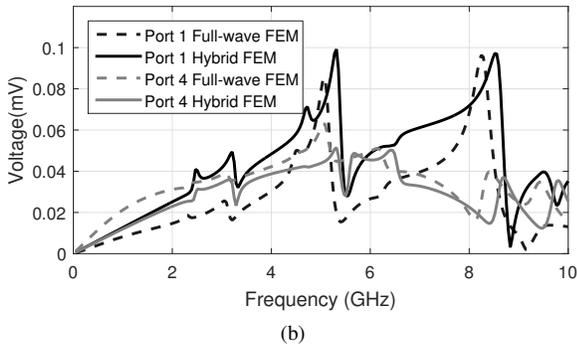
Fig. 3. (a) Two parallel grounded co-planar waveguides separated by a via fence and illuminated by a 1-V/m plane wave polarized in the  $\bar{\theta}$  direction with an incident direction in  $\phi = 45^\circ$ ,  $\theta = 30^\circ$ , (b) voltages induced at Port 1 and Port 4.
