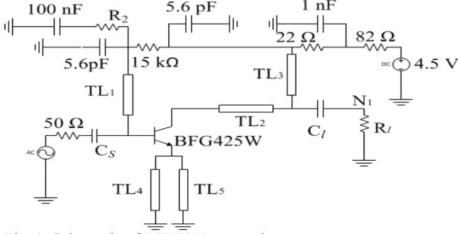
Fig. 1: Schematic of BJT LNA network.
