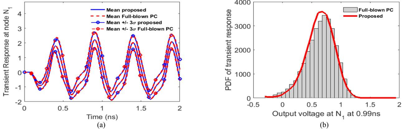
Fig. 2: Statistics of the LNA network of Fig. 1 evaluated using conventional linear regression [5] and the proposed anisotropic HPCE. (a) Statistical analysis of the transient response at node  $N_1$ . (b) Probability distribution function of transient response at node  $N_1$  at  $t = 0.99$  ns.
