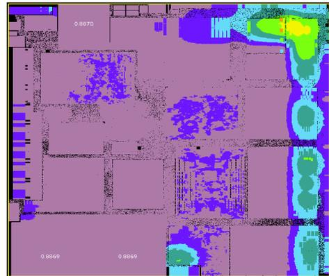
Fig. 5. IR drop map with lumped package model
