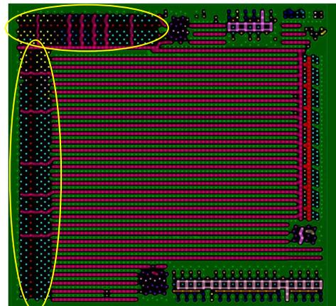
Fig. 6. Package Layout view : shadow region bumps connection
