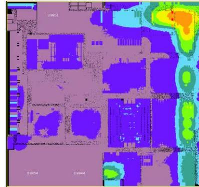
Fig. 10. IR drop map with per-bump model for improved package
