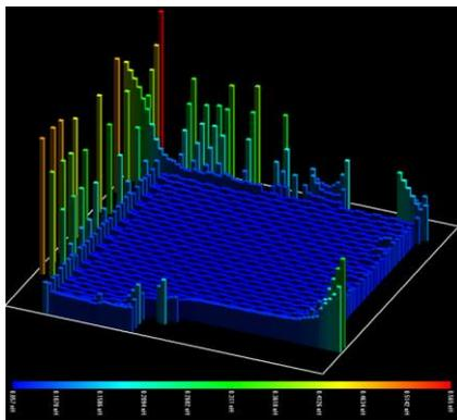
Fig. 7. Core VDD : per-bump package inductance distribution
