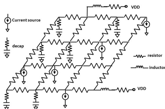
Fig. 1. Chip level power integrity analysis
