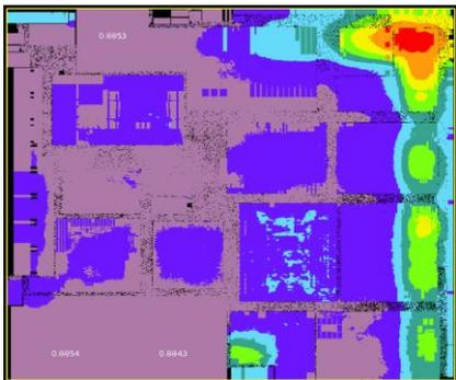
Fig. 8. IR drop map with per-bump package model
