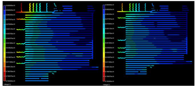
Fig. 9. Package layer1 IR drop contours, before and after improvements
