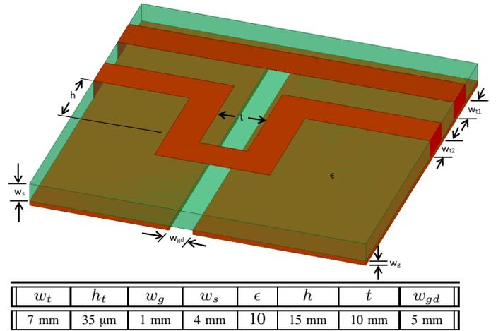
Fig. 1. Four port microstrip line with defective ground structure
