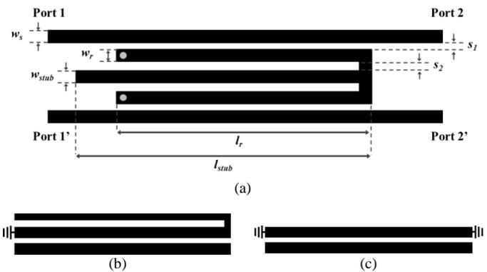
Fig. 1 (a) Proposed layout, equivalent circuits for (b) common mode, and (c) differential mode
