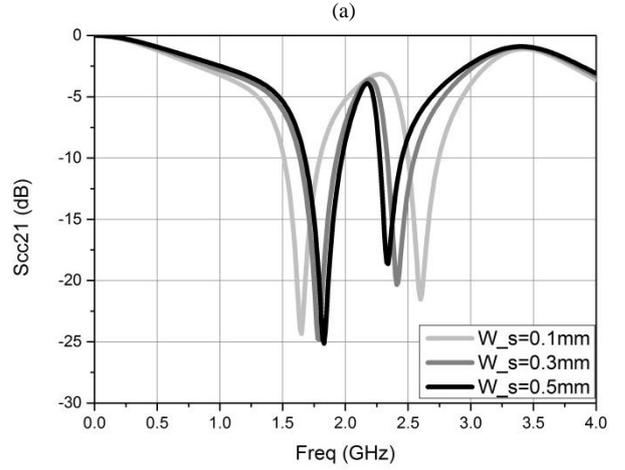
Fig. 4 Variation of  $S_{cc21}$  with (a) different width  $w_o$  and (b) different width  $w_s$ .
