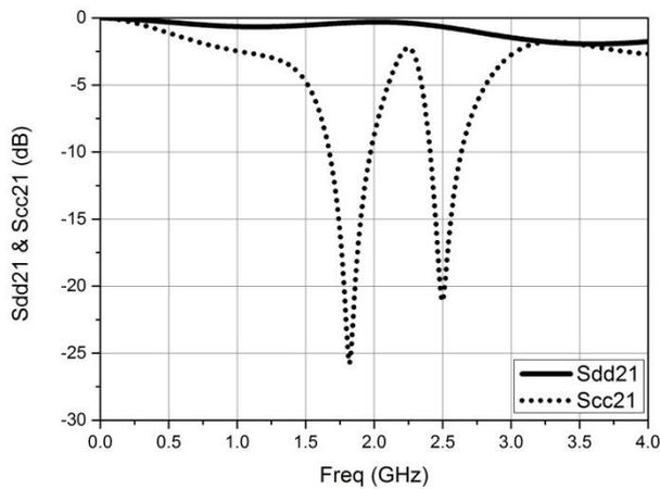
Fig. 5  $S_{cc21}$  &  $S_{dd21}$  of the E-shape resonator dualband common mode filter
