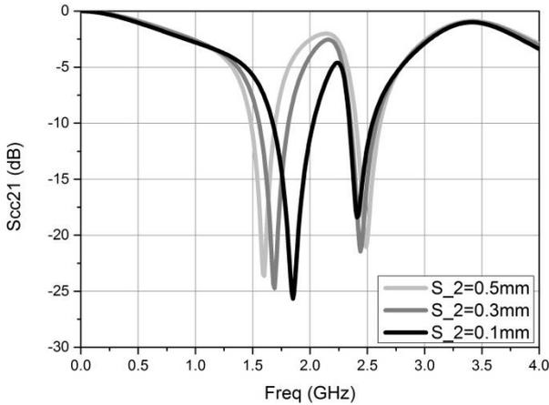
Fig. 3 Variation of  $S_{cc21}$  with different spacing  $s_2$ .
