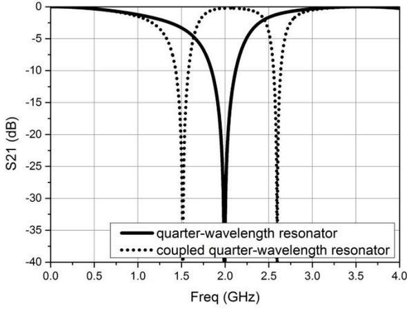
Fig. 2 Comparison between resonance of quarter-wavelength resonator and coupled quarter-wavelength resonator
