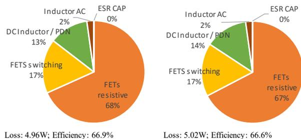
Fig. 4. Left: Loss breakdown and overall efficiency for the 5V:1V conversion at 100 MHz switching frequency. Left: without thermal impact. Right: with thermal impact.
