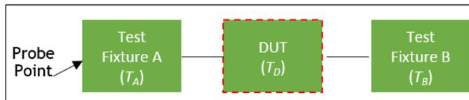
Fig. 2 De-Embedding Approach for DUT in a Test Fixture
