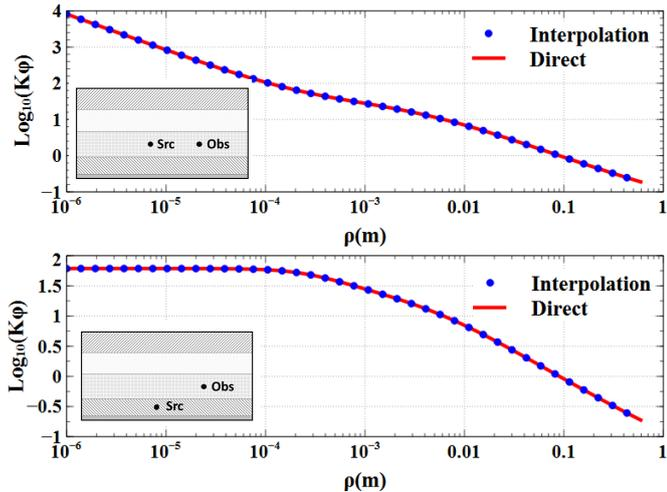
Fig. 2. Comparison between the interpolated and directly calculated scalar potential term: (a) same layer case, (b) adjacent layers case.
