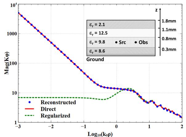
Fig 1. Regularized, direct calculation and reconstructed scalar potential Green's function for the reported four layer stack at 30GHz.
