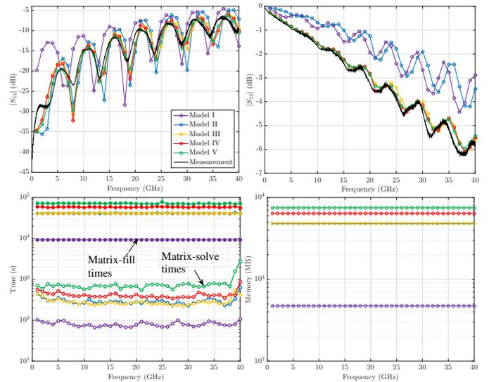
Figure 3. Top:  $S$ -parameters obtained from the five models vs. measured ones. Bottom: Corresponding time and memory costs using a pre-conditioned [13] but unaccelerated iterative MoM solver.
