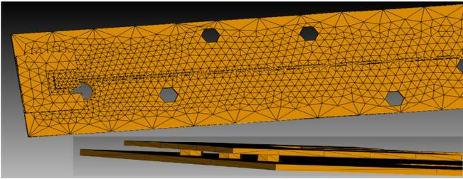
Figure 2. Part of the triangular mesh for model V showing adhesion holes, one of the launchers, conductor side walls, and launcher vias (zoomed view).
