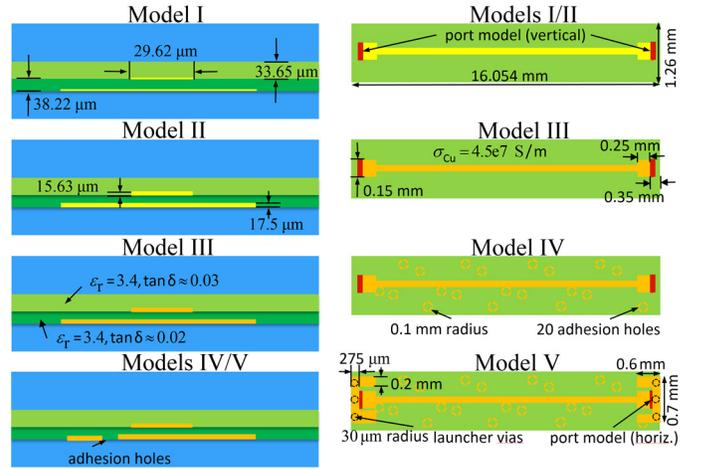
Figure 1. Cross-section (left) and top-down (right) views of the different models for the benchmark problem. (Yellow: PEC; orange: IBC; light green: solder resist; dark green: dielectric substrate; red: port location.)
