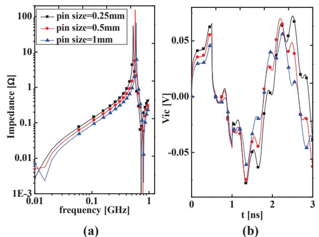
Fig. 5. IC pin size study (a) Results frequency domain solution: Impedance (b) Results time domain solution:  $V_{ic}$
