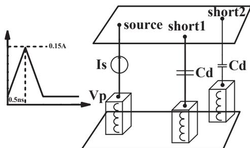
Fig. 1. Current waveform and simplified illustration of PCB model
