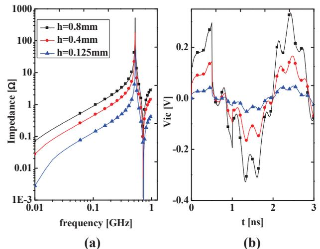
Fig. 6. Impact of different spacings  $h$  for parallel planes (a) Frequency domain result: Impedance (b) Time domain result:  $V_{ic}$
