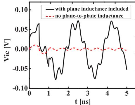
Fig. 4.  $V_{ic}$  of a normal case and ideal case when plane inductance is 0
