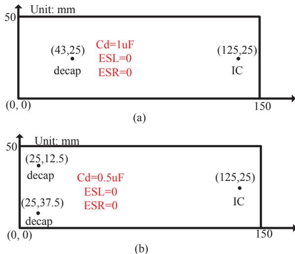
Fig. 7. Decoupling capacitors arrangement (a)case A (b)case B
