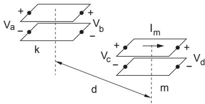
Fig. 3. Coupling between two pairs of overlapping cell pairs.
