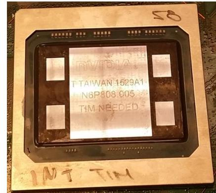
Figure 1: Top view of GPU with four HBM2 chips
