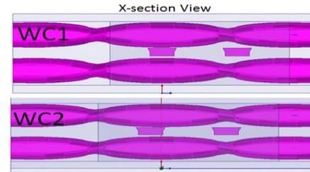
Fig. 3. Two worst case positions for skew for orthogonally routed differential pairs within a PCB dielectric layer having 1ply in the core and prepreg.
