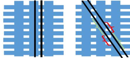
Fig. 2. Diagonal wiring for within differential pair skew mitigation.
