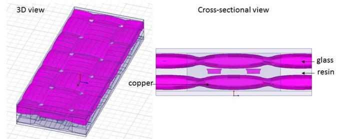
Fig. 1. PCB laminate showing a differential stripline and the glass weaves within the glass-epoxy resin dielectric surrounding.
