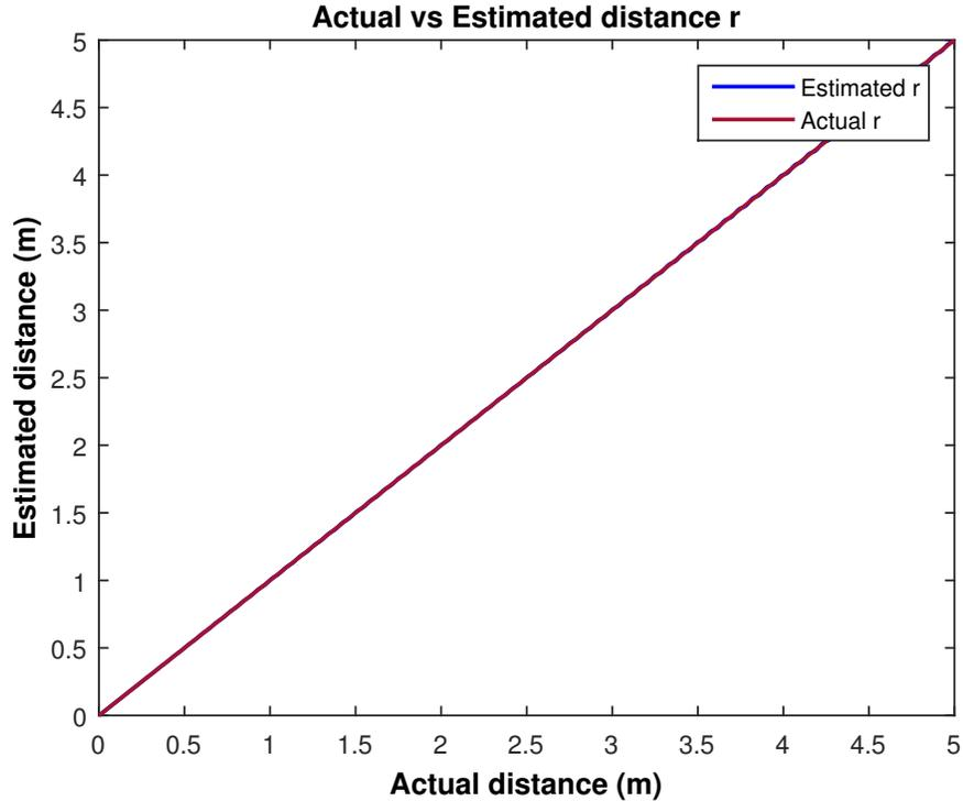
Figure 6.9: Distance Estimation using Two Carrier Frequencies (No Ambiguity)
