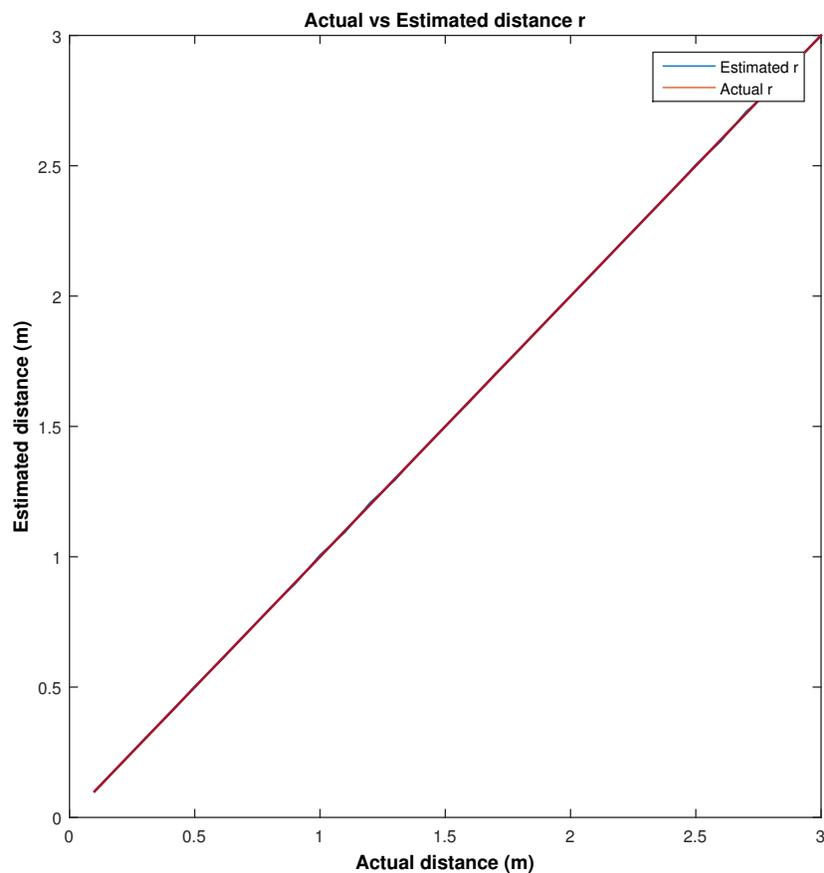
Figure 6.13: Distance Estimation with Correction using PLL
