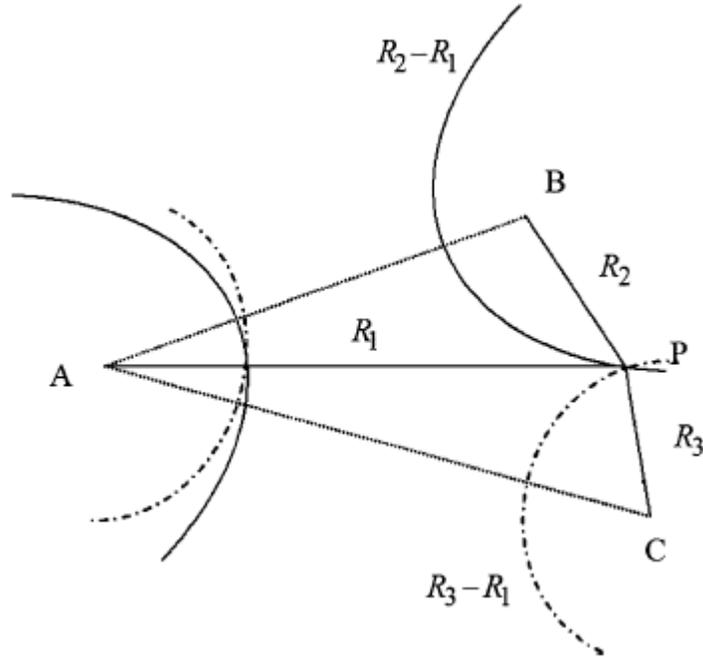
Figure 4.3: TDOA Based Positioning
