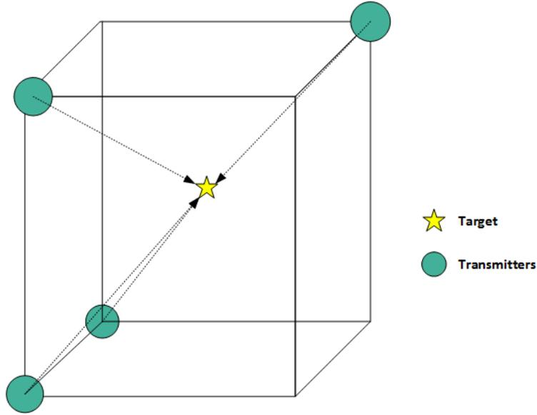
Figure 4.4: Phase of Arrival Based Positioning
