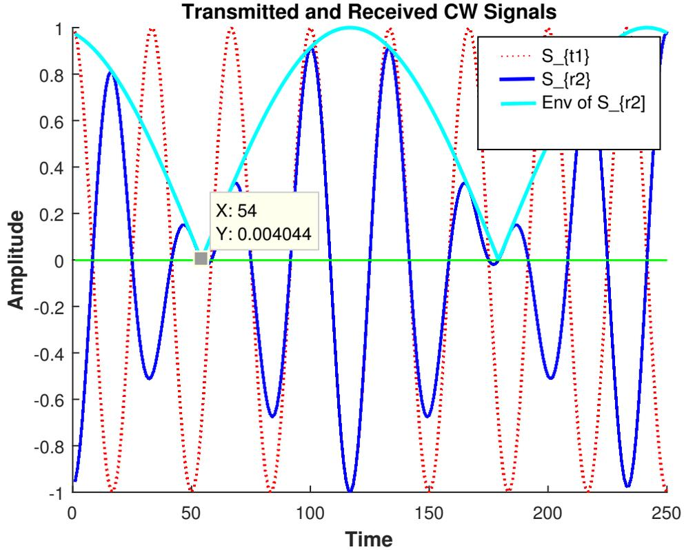
Figure 6.4: Transmitted and Received Signal Waveform for  $r = 0.5 \text{ m}$
