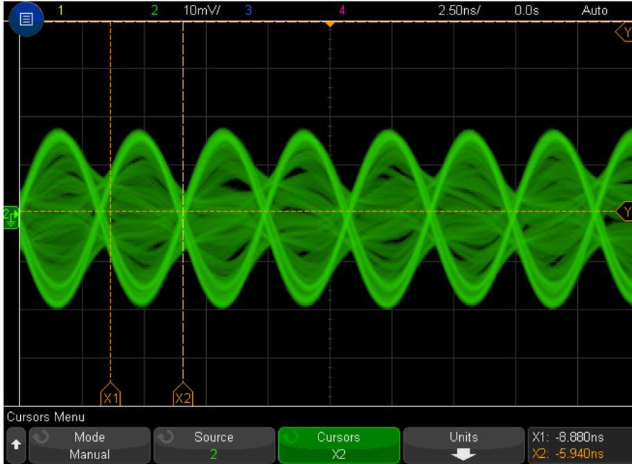
Figure 7.2: Delayed  $S_{r2}$  with a Null at Cursor  $X2=-5.94$  ns
