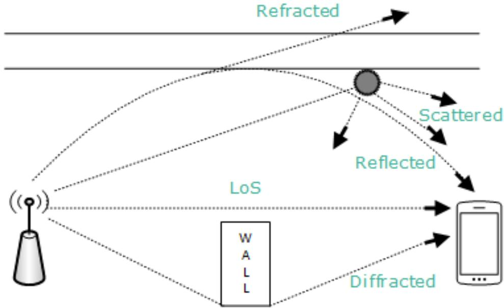
Figure 3.1: Causes of Multipath: Reflection, Refraction, Diffraction and Scattering
