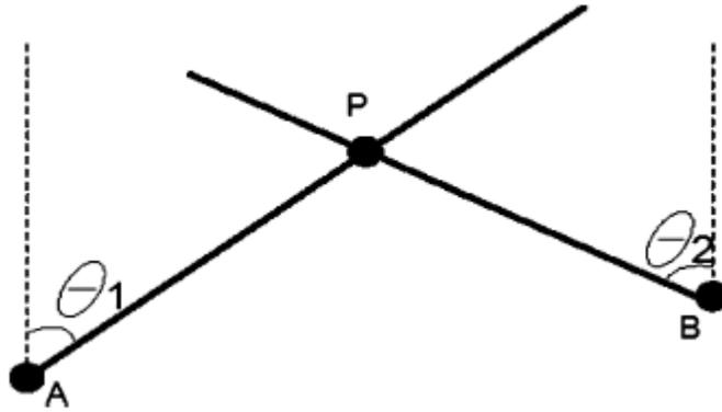
Figure 4.5: Angle of Arrival Based Positioning
