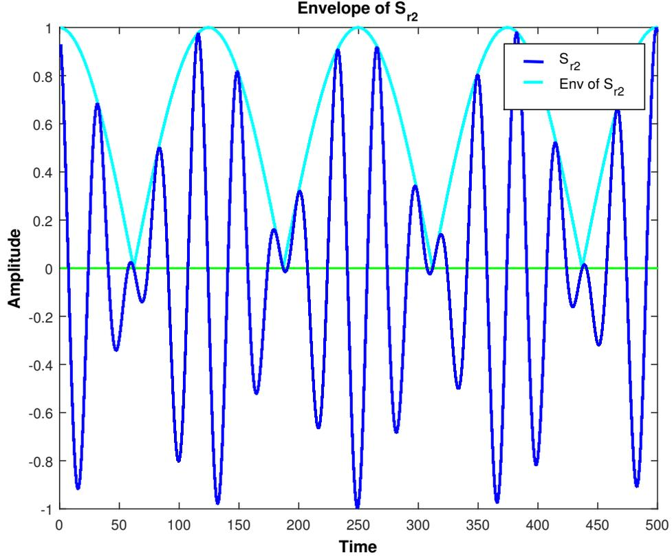
Figure 6.2: Signal  $S_{r2}$  and Its Envelope in Time Domain
