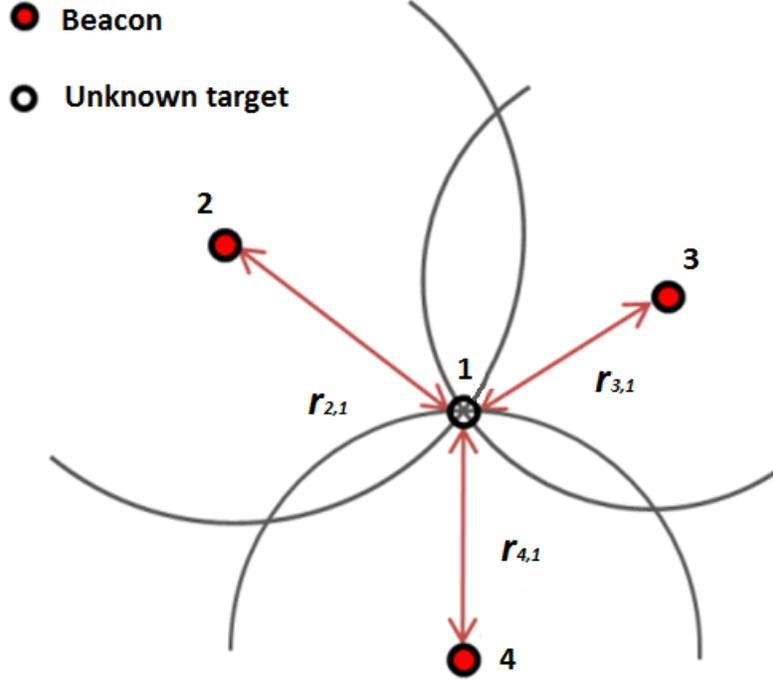
Figure 5.2: Location Estimation using Trilateration
