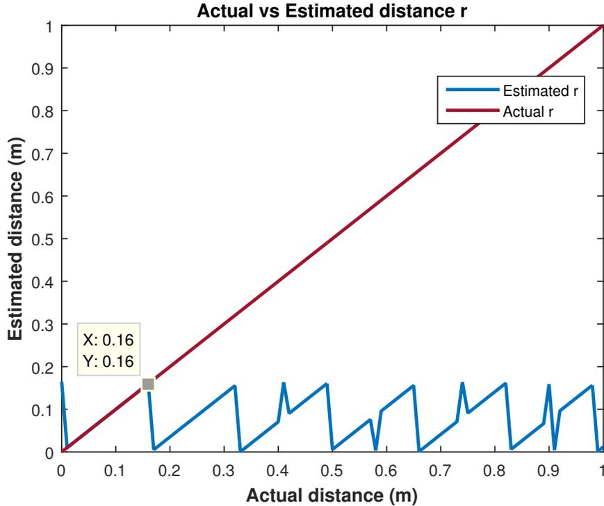
Figure 6.7: Distance Estimation with Single Carrier Frequency
