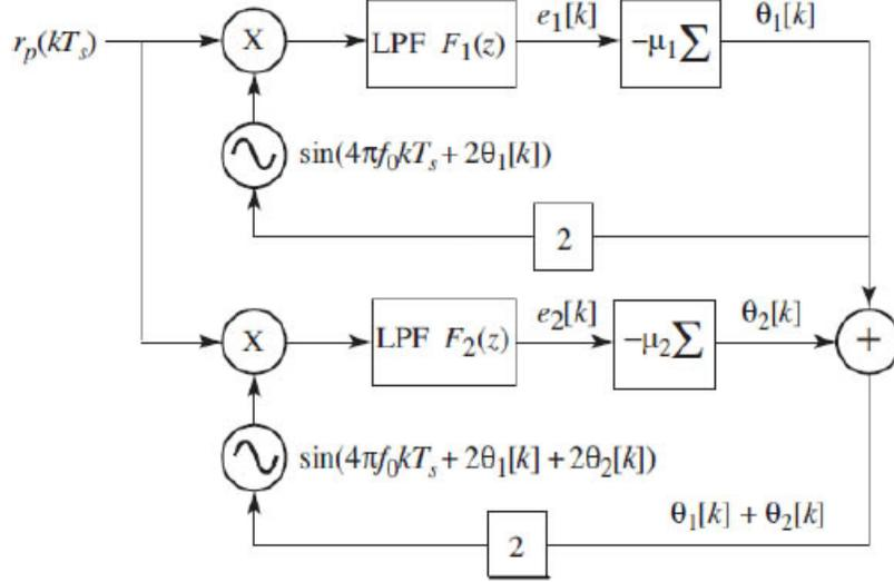
Figure 6.10: The Dual Phase Locked Loop Structure
