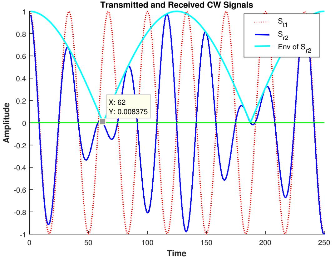
Figure 6.3: Received Signal Waveform for  $r = 0$  m
