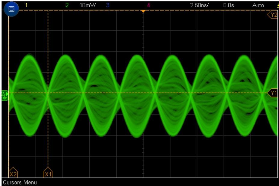
Figure 7.1:  $S_{r2}$  with a Null at Cursor  $X1 = -8.880$  ns
