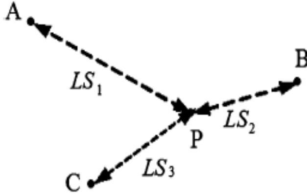
Figure 4.2: RSSI Based Positioning
