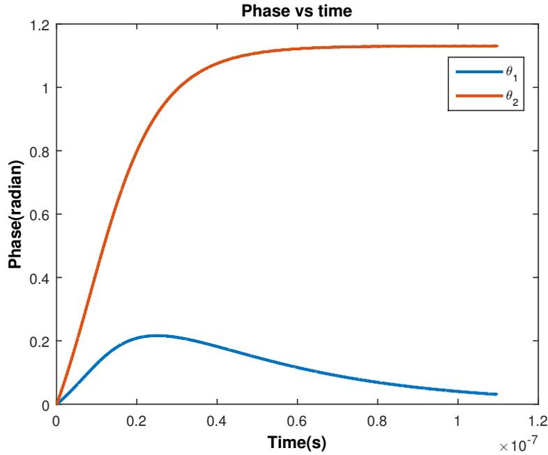
Figure 6.11: Convergence Function of a Dual PLL
