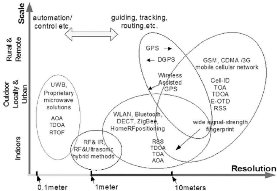
Figure 2.1: Overview of Wireless Positioning Systems
