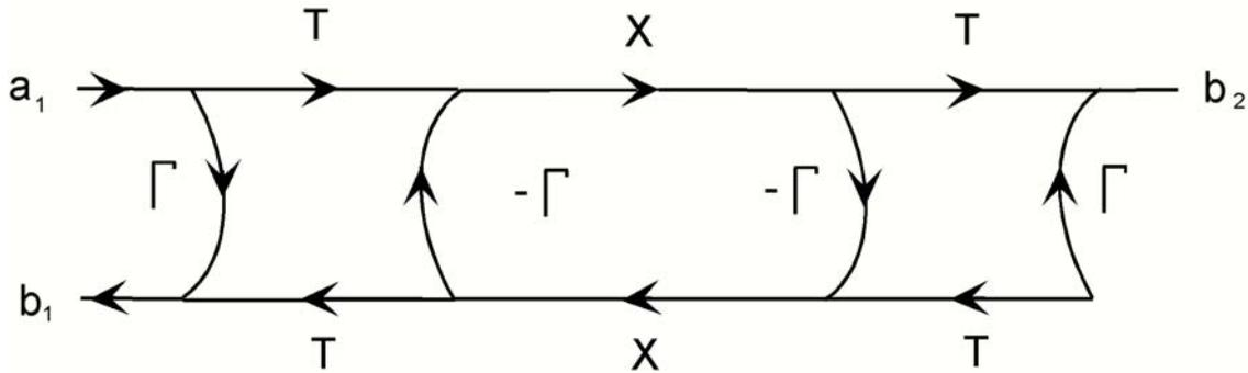
Figure 3.3 Transmission line flow graph.
