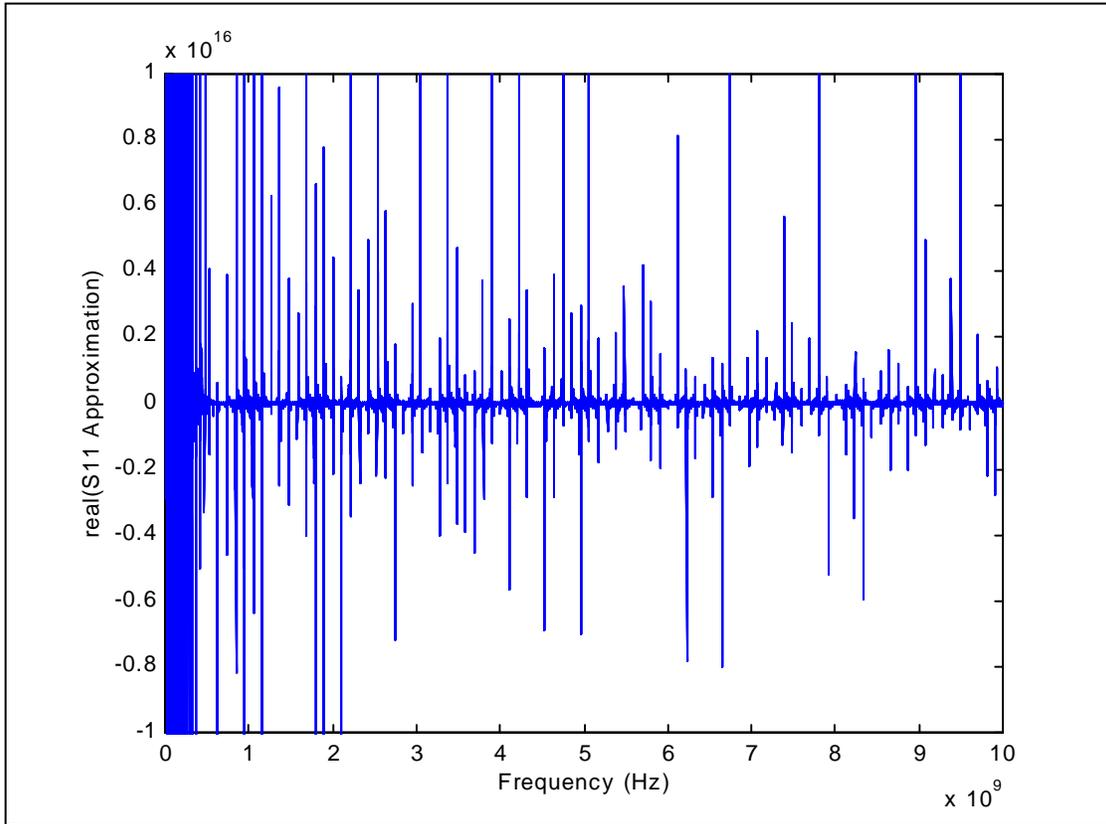
Figure 3.6 Real component of  $S_{11}$  approximation versus frequency.
