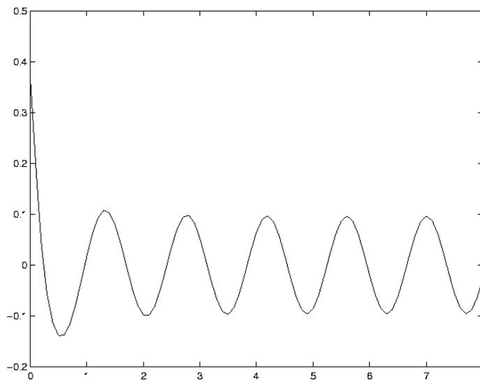
Figure 3.1 Transmission line transfer function versus frequency.
