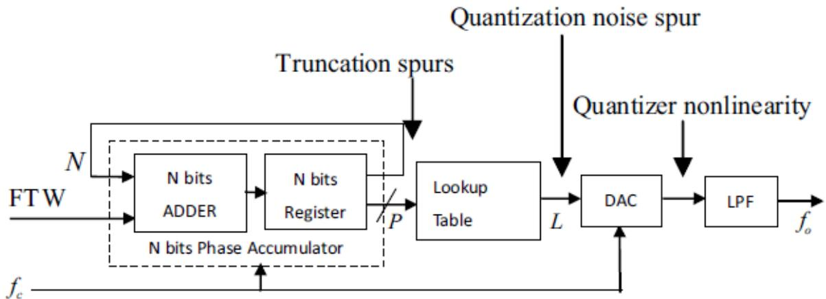
Figure 2.1: Basic Structure of Direct Digital Synthesizer [3]
