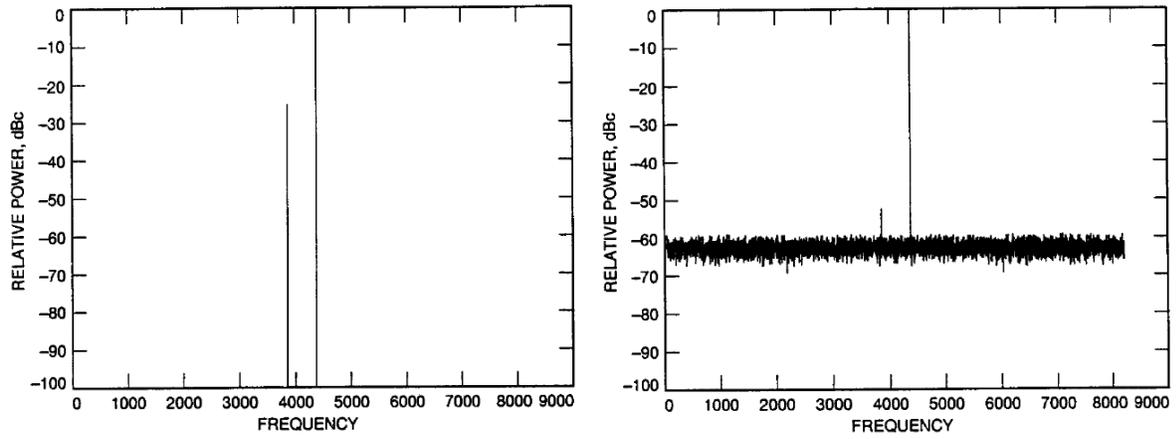
Figure 4.4: Power spectrum of 5-bit phase truncated sine wave without dithering (Left) and with dithering (Right) [6]
