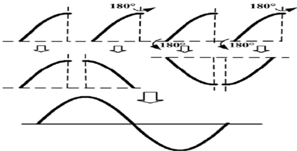
Figure 3.1: Logic behind forming Sine Wave
