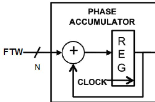
Figure 2.2: Phase Accumulator [3]
