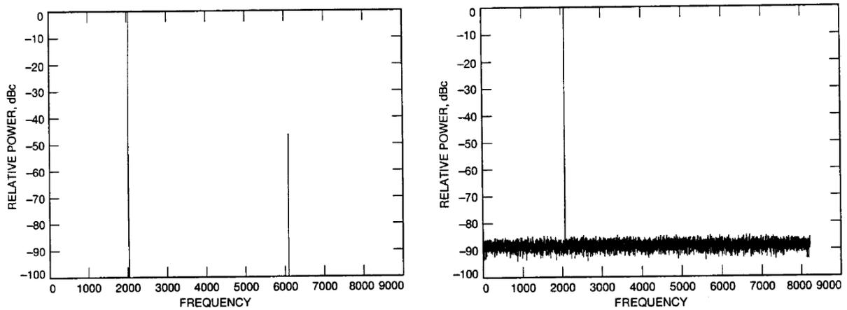
Figure 4.5: Power spectrum of 8-bit phase truncated sine wave without dithering (Left) and with dithering (Right) [6]
