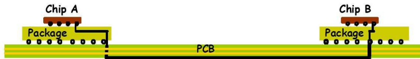
Figure 6.15 Chip-to-chip interconnect system that has up to 12-in long FR4 PCB traces and two packages with up to 20-mm long traces.
