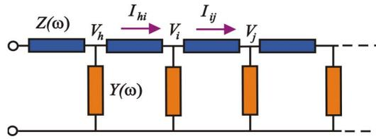
Figure 3. Model of an interconnect with frequency-dependent parameters
