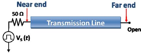
Figure 4. Transmission line configuration used in the simulation
