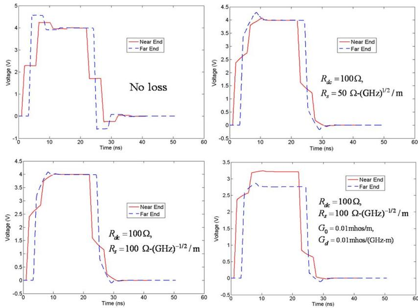
Figure 5. Shape of the pulse at the near and far ends of the line
