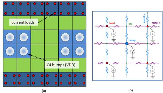
Figure 3. Model structure for IR drop analysis
