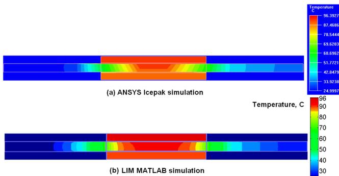
Figure 9. Temperature distribution within the structure (cross-section)
