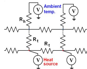
Figure 6. Thermal-electrical model structure
