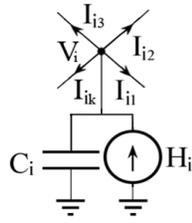
Figure 2. LIM node equivalent circuit.
