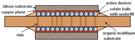
Figure 8. System of two chips with an interposer substrate
