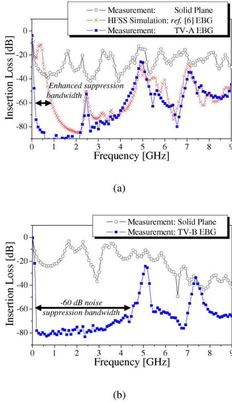
Fig. 3. (a)  $|S_{21}|$  responses of TV-A EBG PDN. 3 and (b).  $|S_{21}|$  responses of TV-B EBG PDN.
