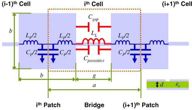
Fig. 1. One-dimensional equivalent circuits of EBG PDN.
