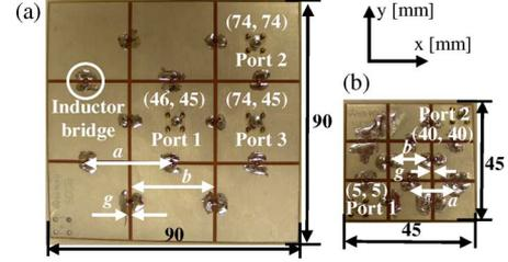
Fig. 2. Fabricated EBG PDNs: (a) TV-A and (b) TV-B.
