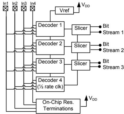
Figure 3. Proposed receiver architecture for modal signaling
