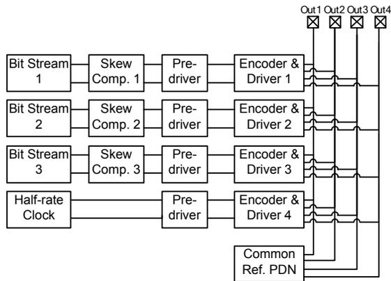
Figure 2. Proposed transmitter architecture for modal signaling
