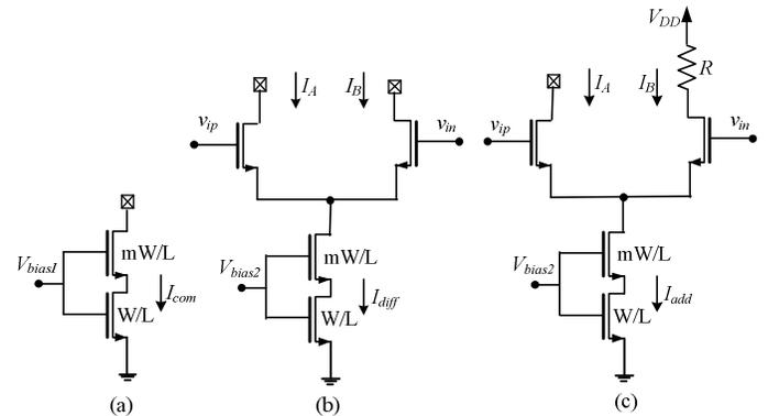
Figure 4. (a) Open-drain drivers producing the common-voltage levels; (b) Current-steering for shared currents, and (c) for non-shared currents
