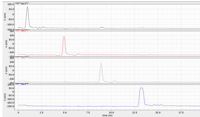
Figure 6. Unit pulse responses of signals over equivalent modal channels
