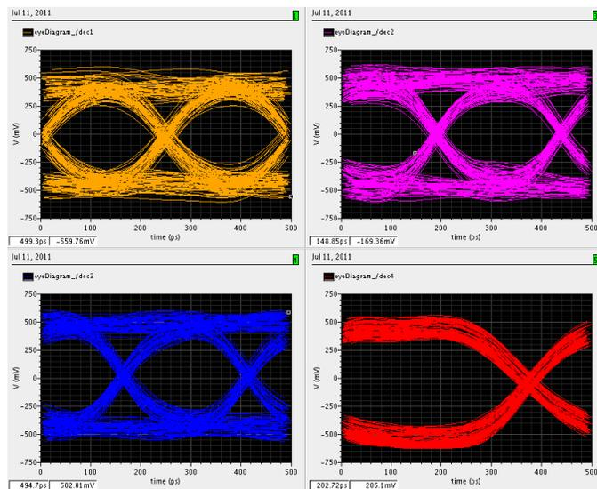
Figure 7. Eye diagrams of decoded modal signals (normalized to  $1V_{pp}$ )
