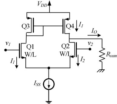
Figure 5. Current subtractor for modal decoder realization
