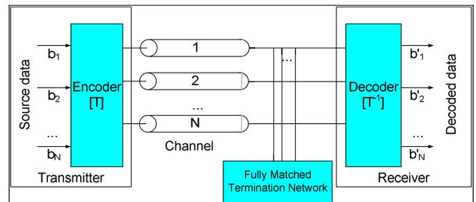
Figure 1(a). Block diagram of modal signaling system components
