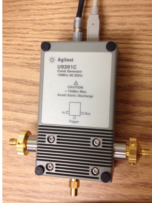
Figure 3.3: Repetitive-pulse generator (also referred to as a comb generator) that serves as a phase reference for cross-frequency phase measurements.
