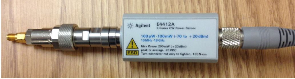
Figure 3.2: This power meter is used to measure the absolute power being sourced by the PNA-X. Unlike linear PNA-X measurements which leverage the linear property of homogeneity and measure the ratio of scattered to incident waves, all nonlinear PNA-X measurements require an amplitude calibration because these measurements are nonratioed.
