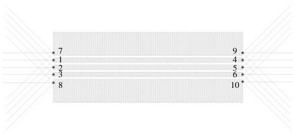
Figure 4.15 Three-coupled coplanar layout (not to scale) with port numbers.
