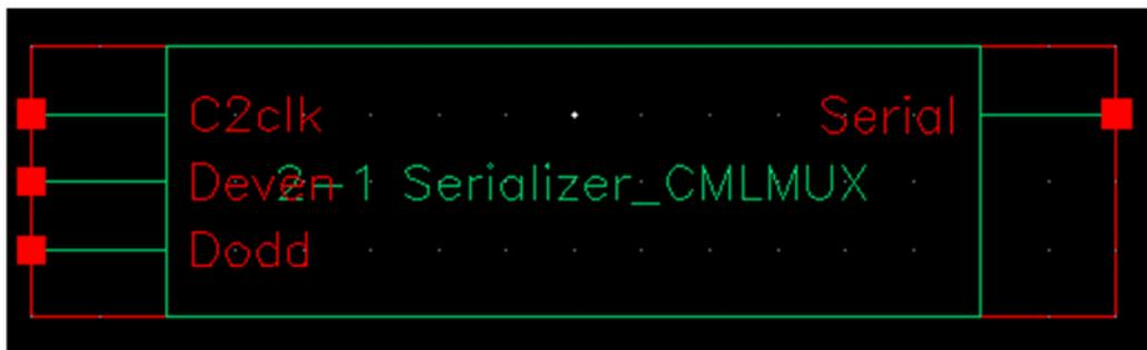
Figure 4.24 Symbol of the entire 2:1 Serializer circuit
