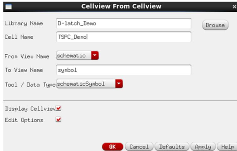
Figure 4.17 Create a symbol from schematic
