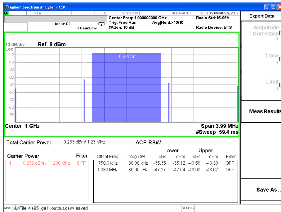
Figure 7.3: Gali-1+ ACP under NB-CDMA Digital Modulated Input Signal at -10 dBm
